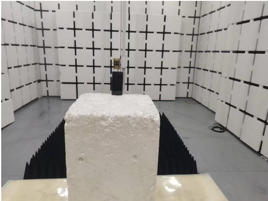
Set-up for Radiated Spurious Emission, Above 1GHz
