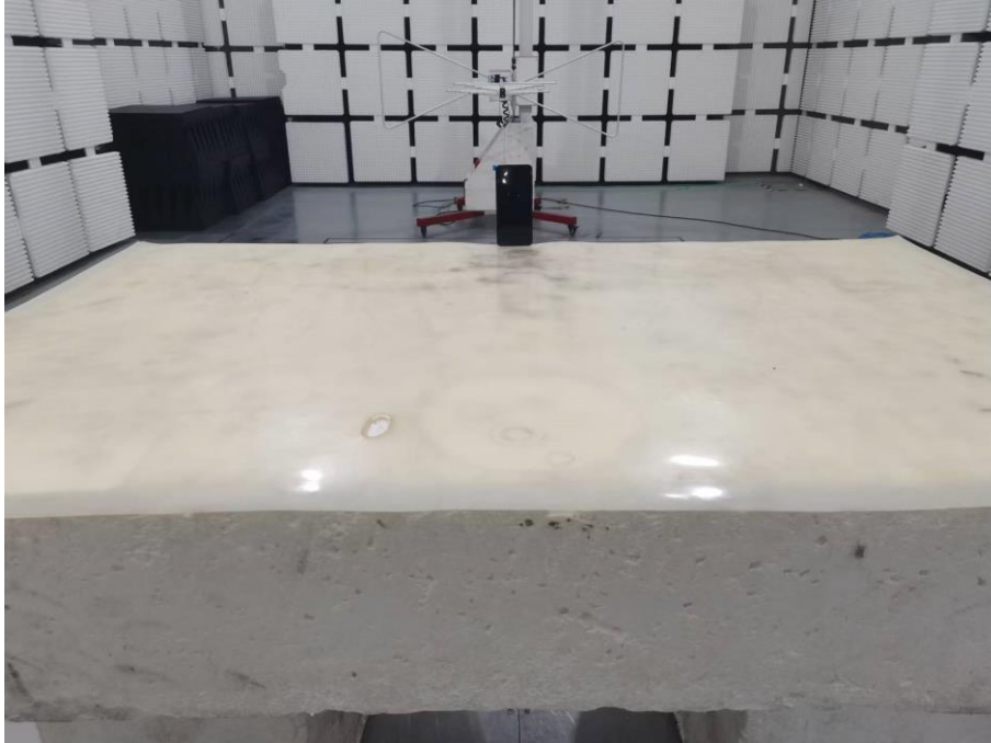
Set-up for Radiated Spurious Emission, Above 1GHz
