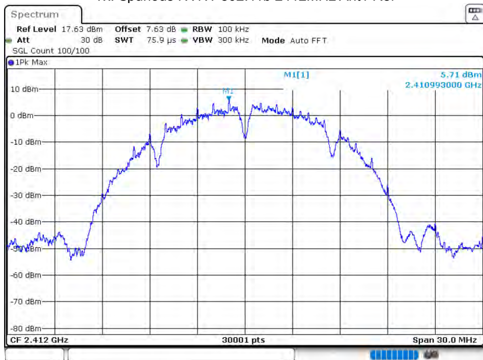
Tx. Spurious NVNT 802.11b 2412MHz Ant1 Ref
