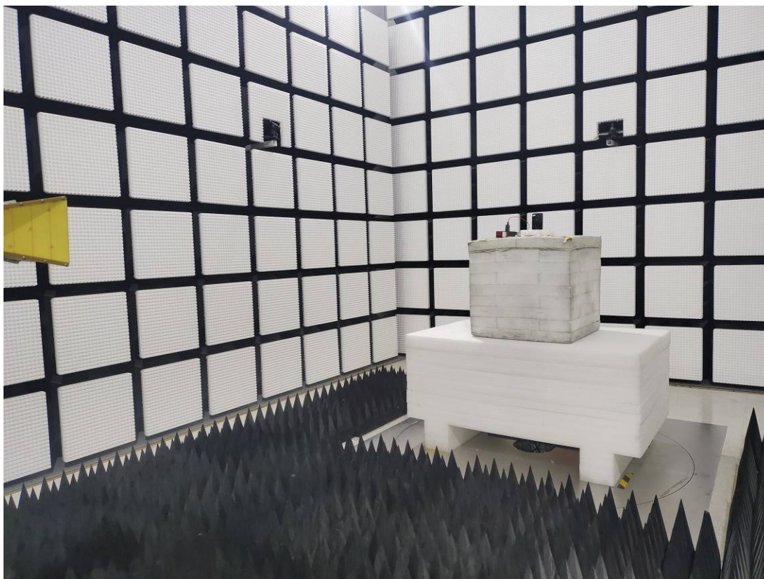
Radiated Emission Above 1GHz View
