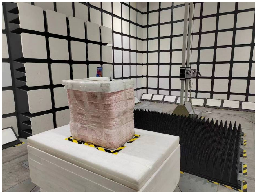
Radiated Emissions View (Above 1 GHz) – TX
