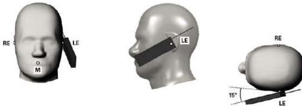
Fig.11.4 Illustration for Tilted Position
