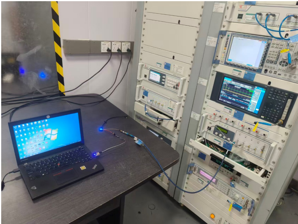
Connect EUT antenna terminal test
