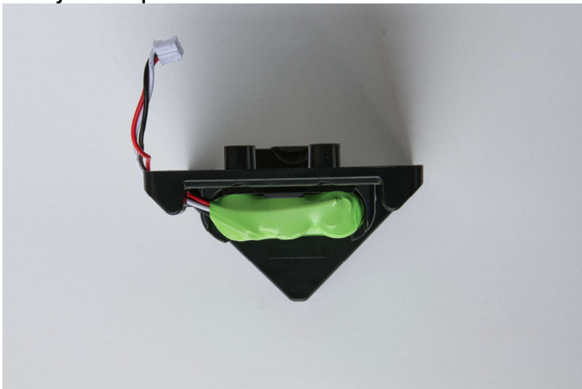
Battery Pack Top View
