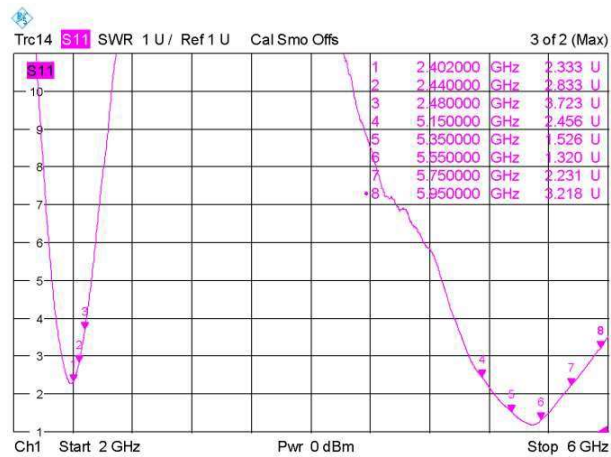
Figure 5-3 VSWR Renesas RRQ610x1-008 Wi-Fi module antenna. Module in middle position.
