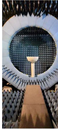
Figure 5-5 Satimo SG-23 6 GHz Stargate Antenna Test Chamber.
