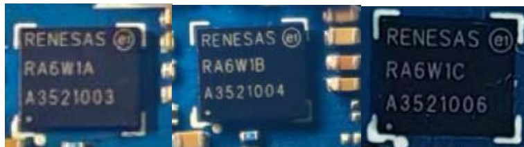
Figure 1. IC marking on the RA6W1 family members
