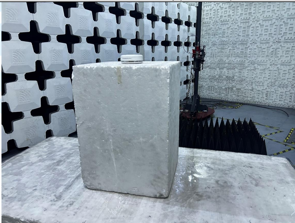
Radiated emission Test Setup (Above 1 GHz)
