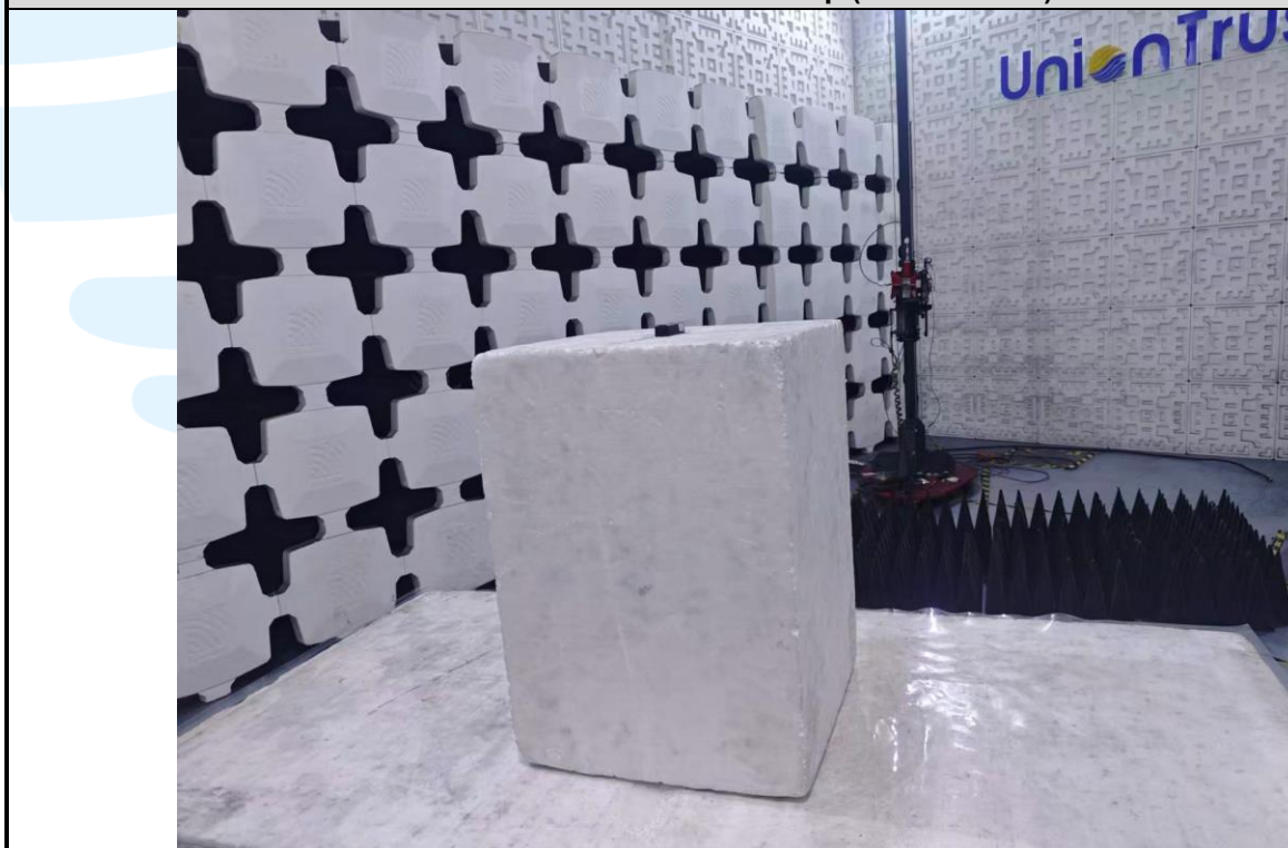
Radiated emission Test Setup (Above 1 GHz)
