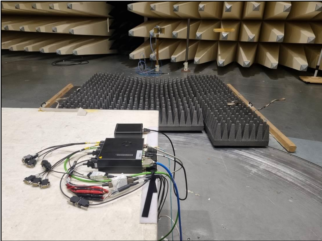
Photo 3: setup of radiated emission >1 GHz
