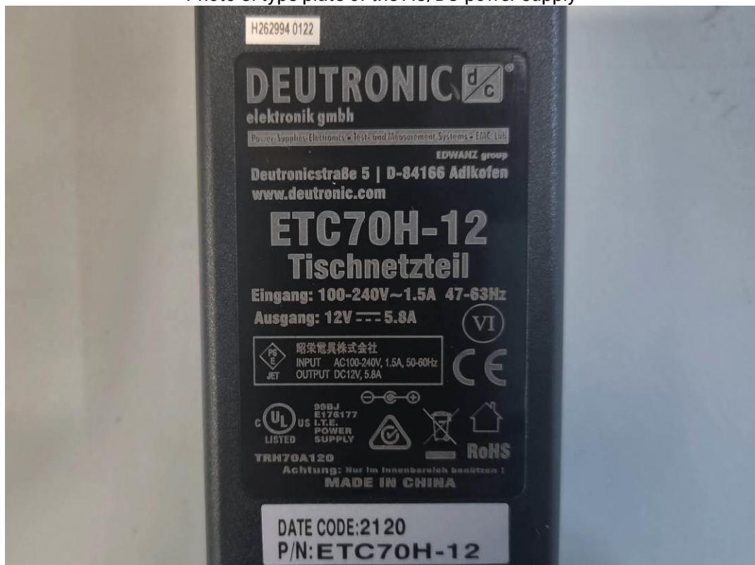
Photo 8: type plate of the AC/DC-power supply
