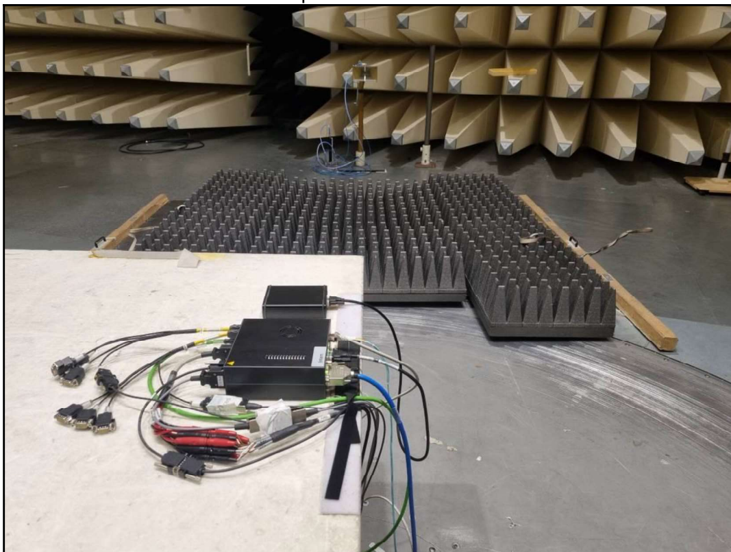
Photo 3: setup of radiated emission >1 GHz
