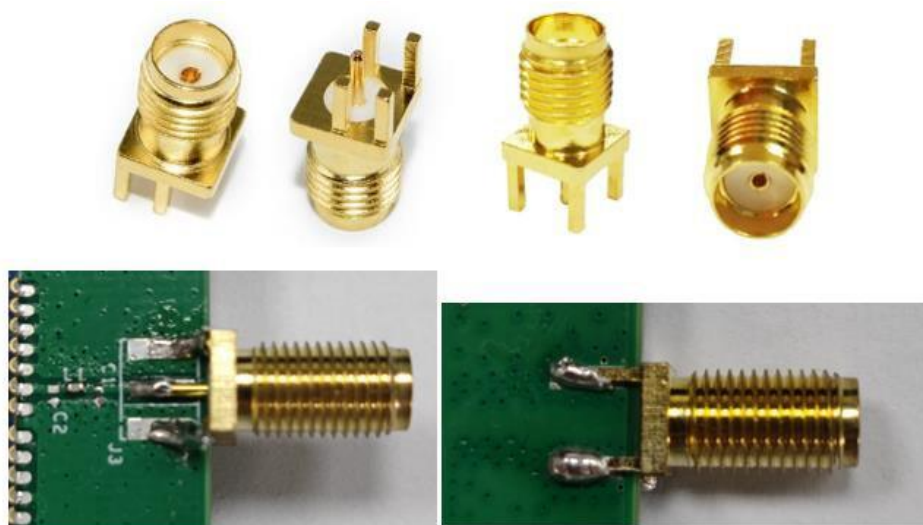
Figure 27 Common SMA coaxial connectors
