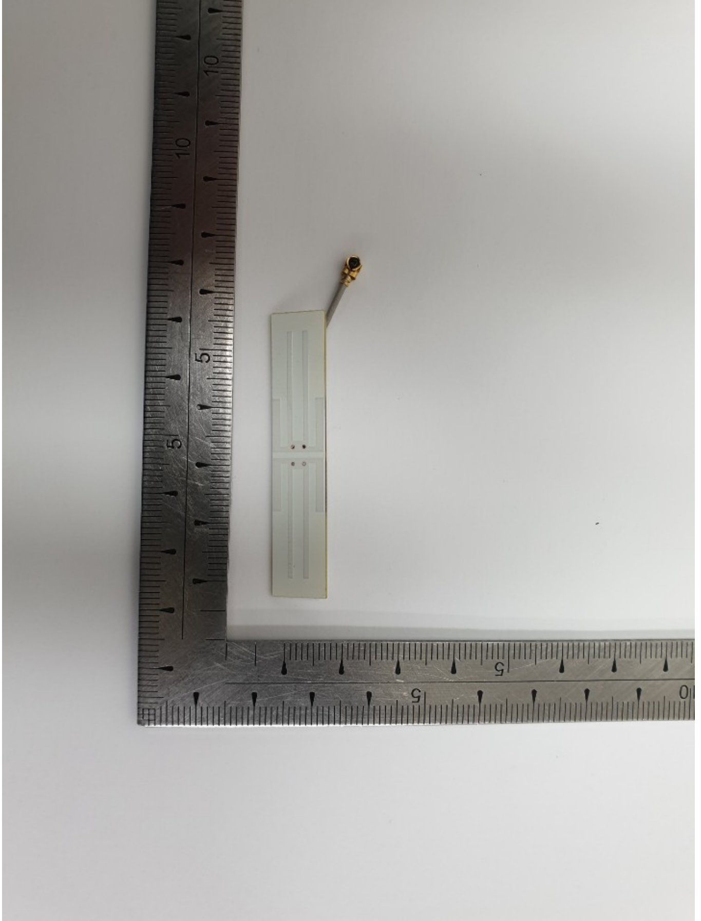
Antenna 2 (Additional) / PCB Antenna [Model name: AEi-2450/5500P-IPEX35]
