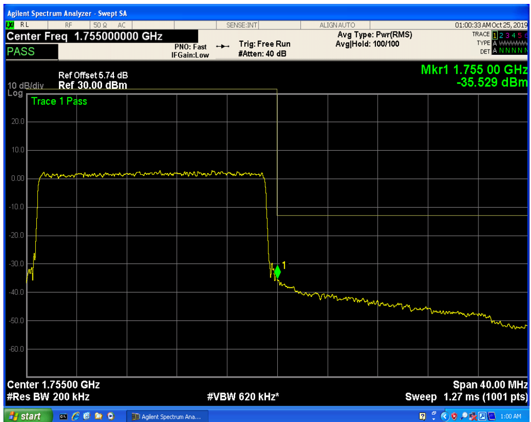
LTE Band4 QAM16 BW=20MHz Channel=20300 RB Size=1 Position=#0
