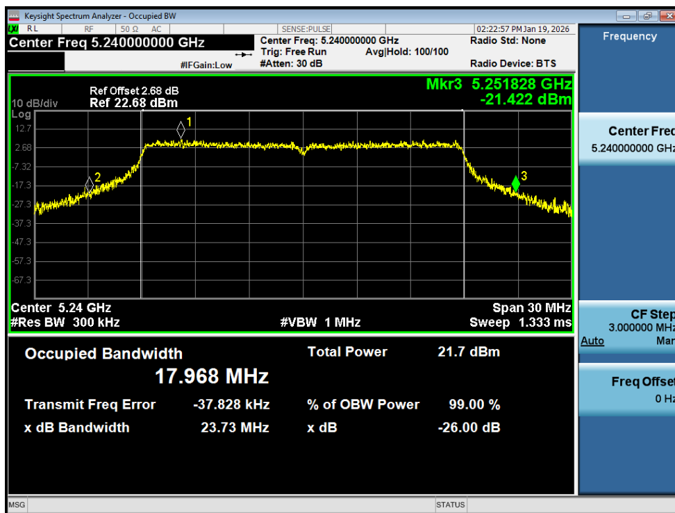
-26dB Bandwidth NVNT n20 5240MHz Ant1
