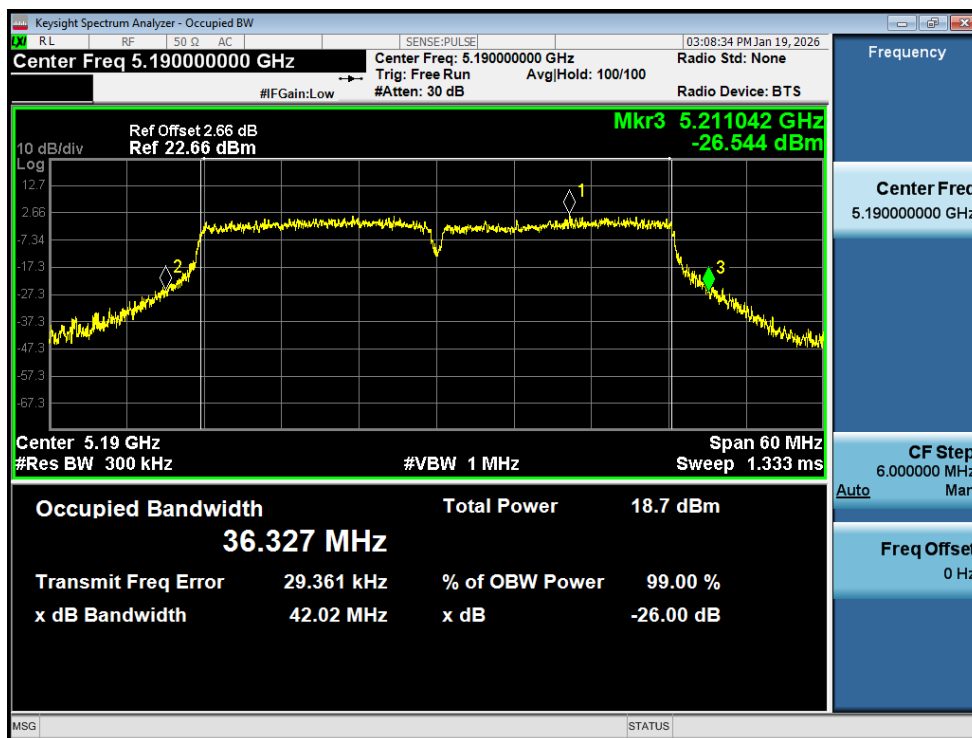
-26dB Bandwidth NVNT ac40 5190MHz Ant2
