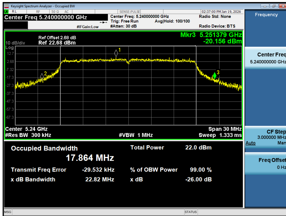
-26dB Bandwidth NVNT ac20 5240MHz Ant1
