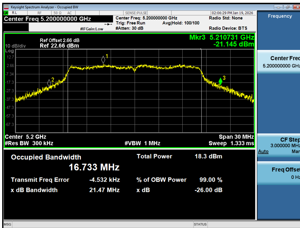
-26dB Bandwidth NVNT a 5200MHz Ant2
