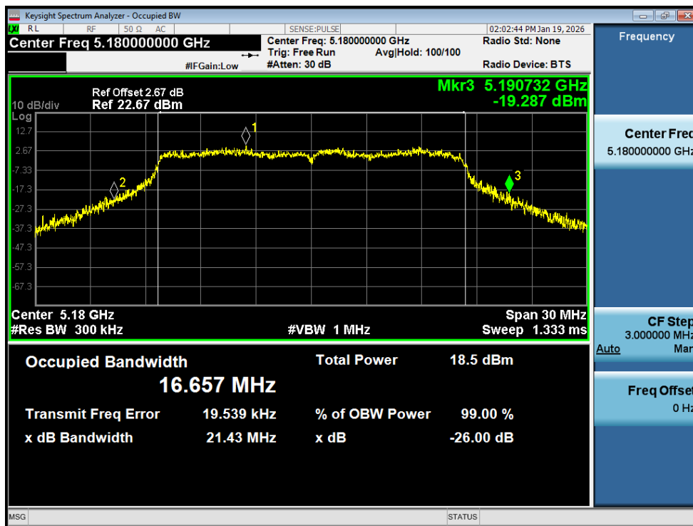
-26dB Bandwidth NVNT a 5180MHz Ant2
