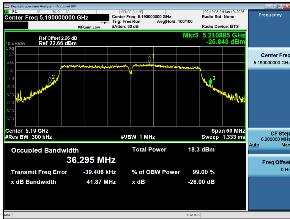
-26dB Bandwidth NVNT n40 5190MHz Ant2
