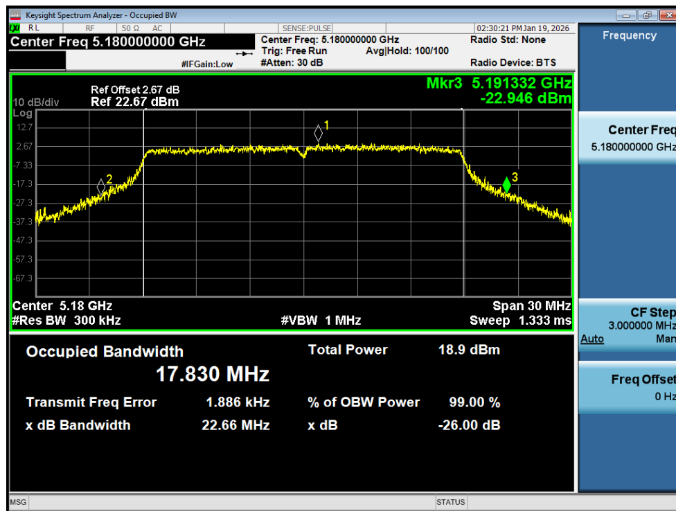
-26dB Bandwidth NVNT ac20 5180MHz Ant2
