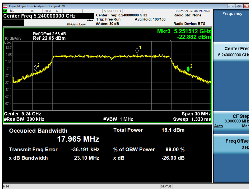
-26dB Bandwidth NVNT n20 5240MHz Ant2
