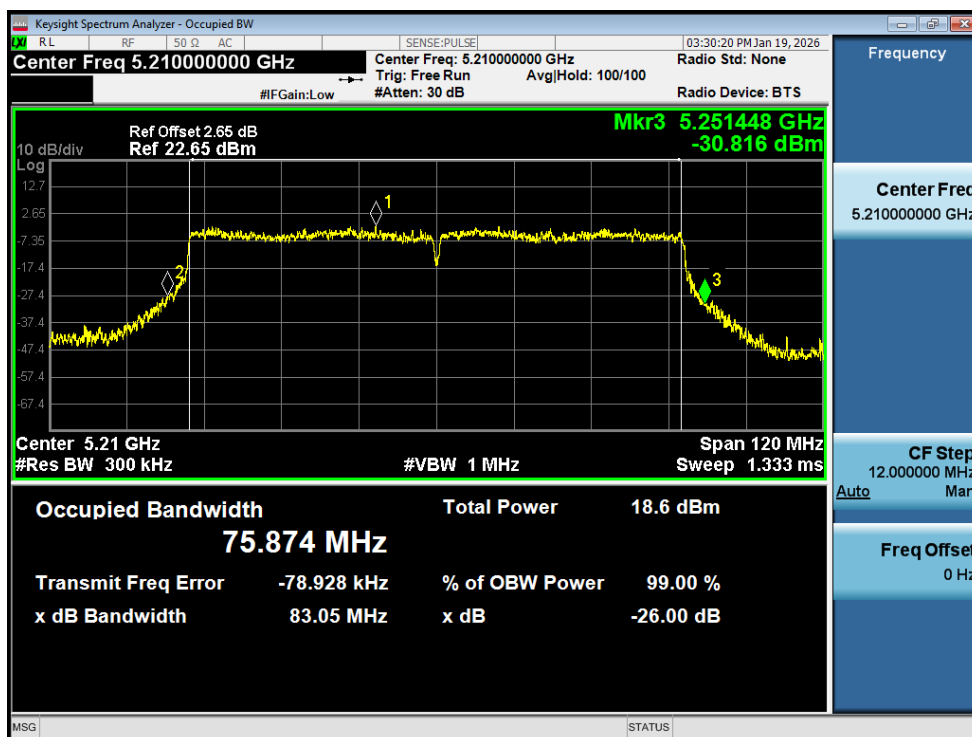
-26dB Bandwidth NVNT ac80 5210MHz Ant2
