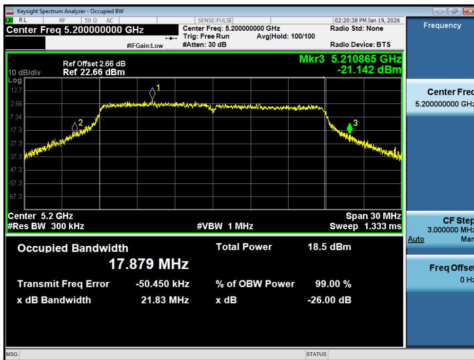
-26dB Bandwidth NVNT n20 5200MHz Ant2
