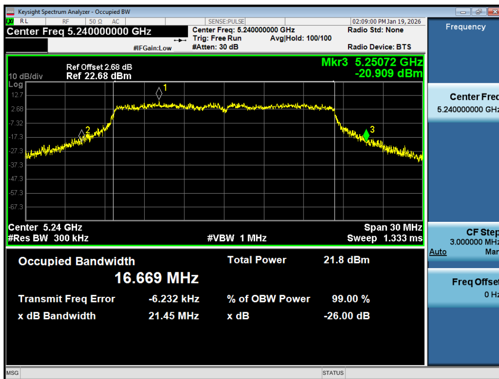
-26dB Bandwidth NVNT a 5240MHz Ant1
