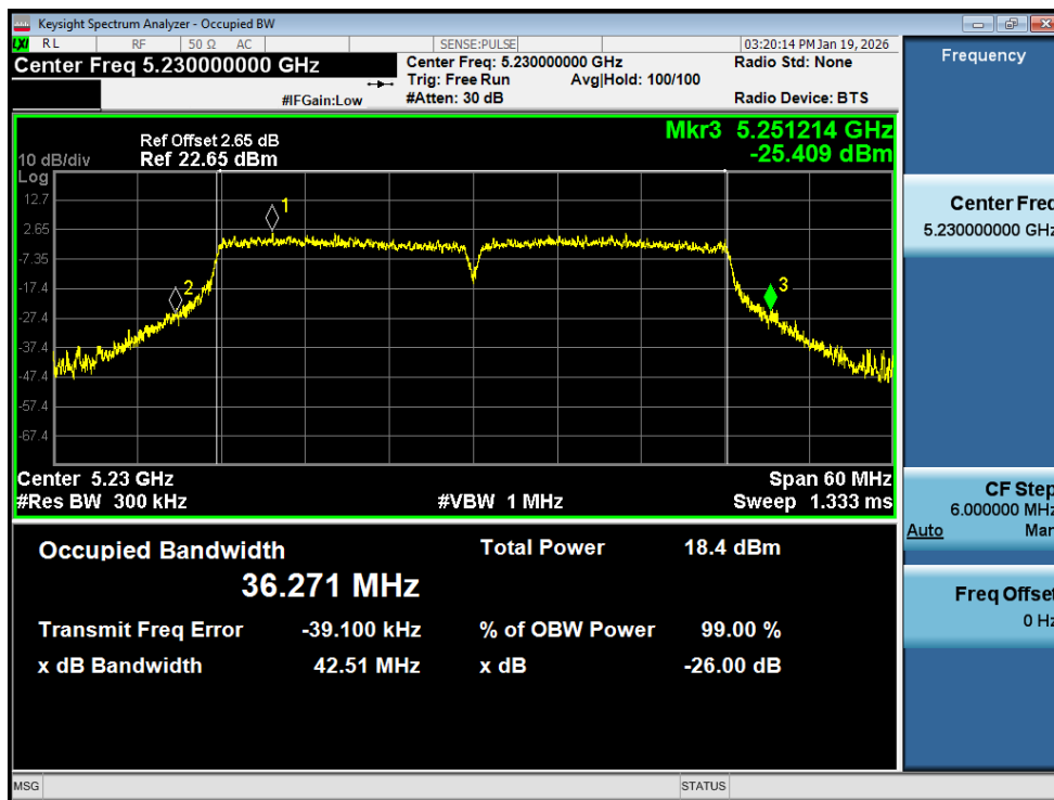
-26dB Bandwidth NVNT ac40 5230MHz Ant2
