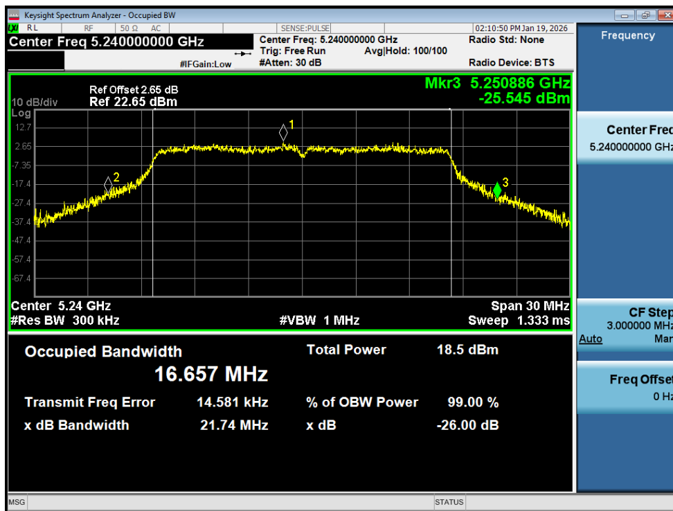
-26dB Bandwidth NVNT a 5240MHz Ant2
