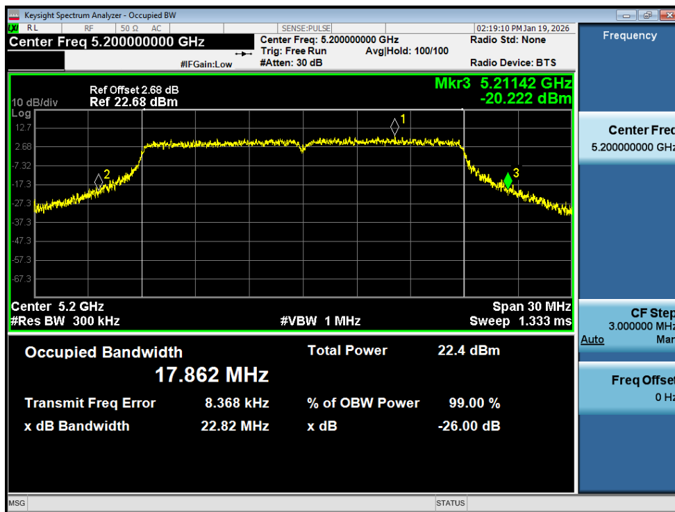
-26dB Bandwidth NVNT n20 5200MHz Ant1
