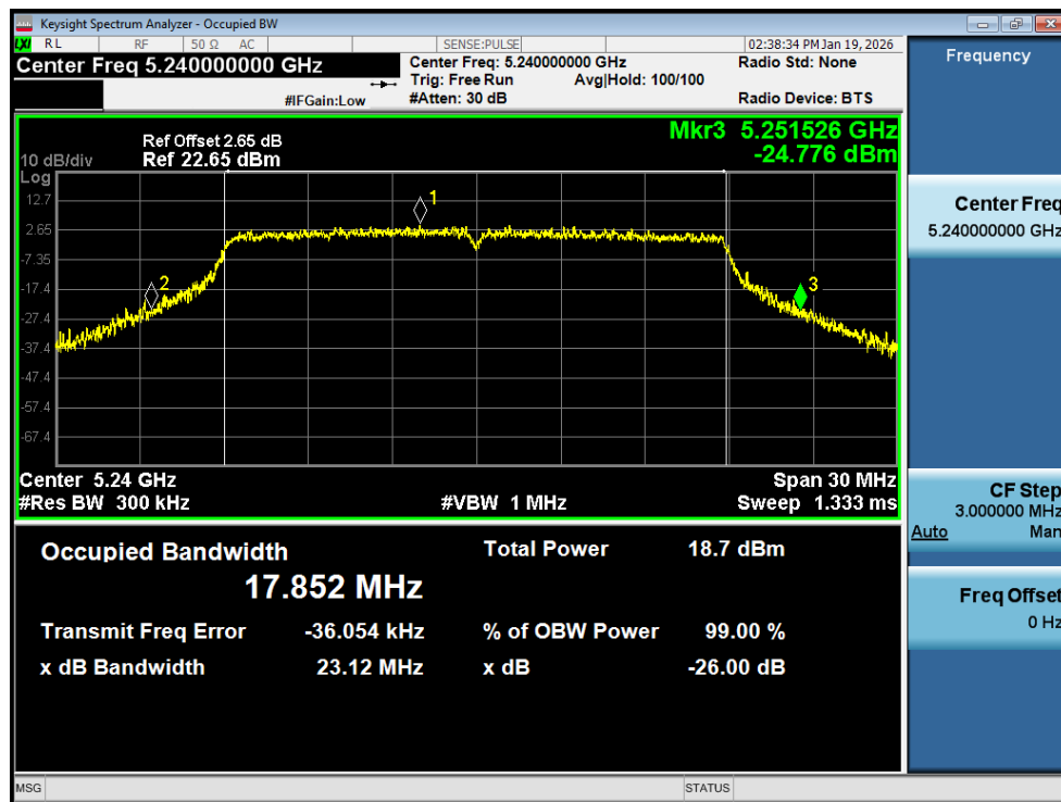
-26dB Bandwidth NVNT ac20 5240MHz Ant2
