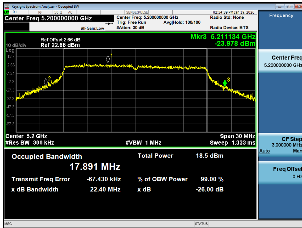
-26dB Bandwidth NVNT ac20 5200MHz Ant2
