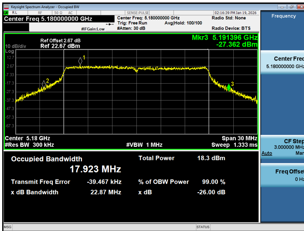
-26dB Bandwidth NVNT n20 5180MHz Ant2
