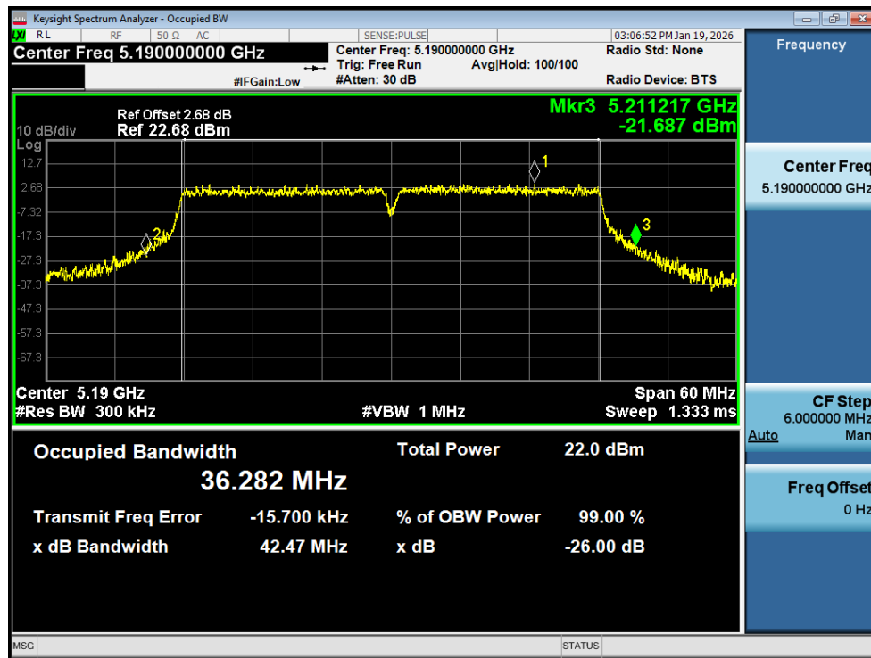
-26dB Bandwidth NVNT ac40 5190MHz Ant1
