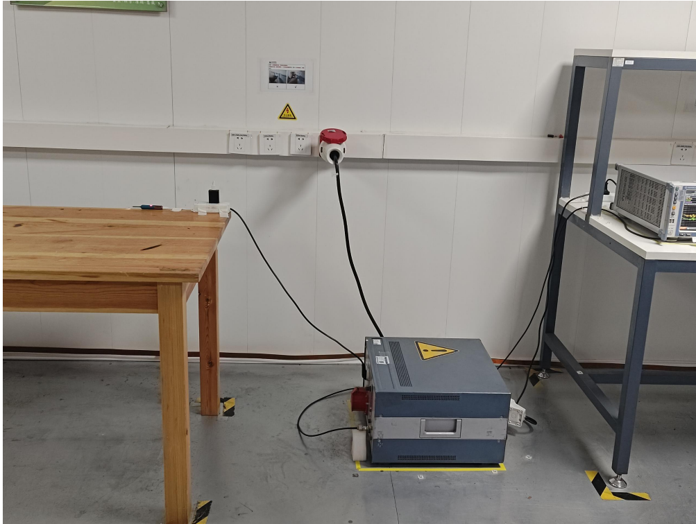
Test Setup Photo(s) of Conducted Emissions Measurement
