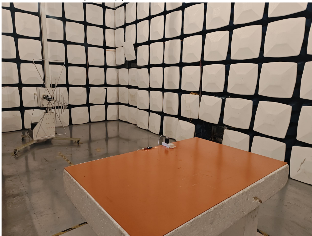
Test Setup Photo(s) of Radiated Emissions Measurement
