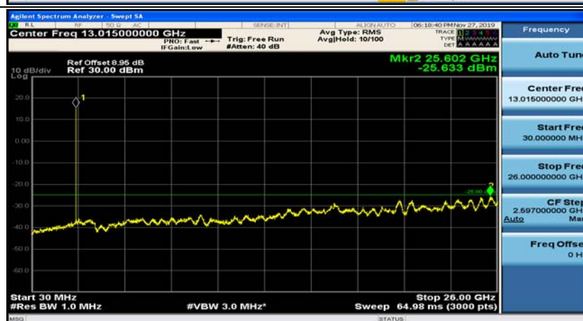
(Channel Bandwidth: 5 MHz)_LCH_16QAM_1RB#12
