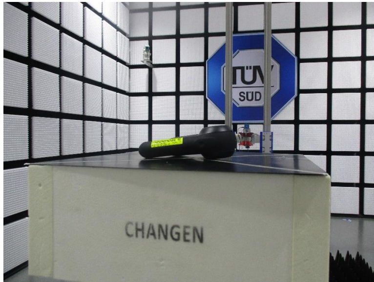
Test Setup – Spurious emissions (1000-18000 MHz)
