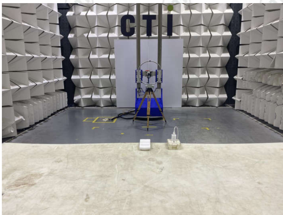
Radiated spurious emission Test SetupRX-4(Below 30MHz)
