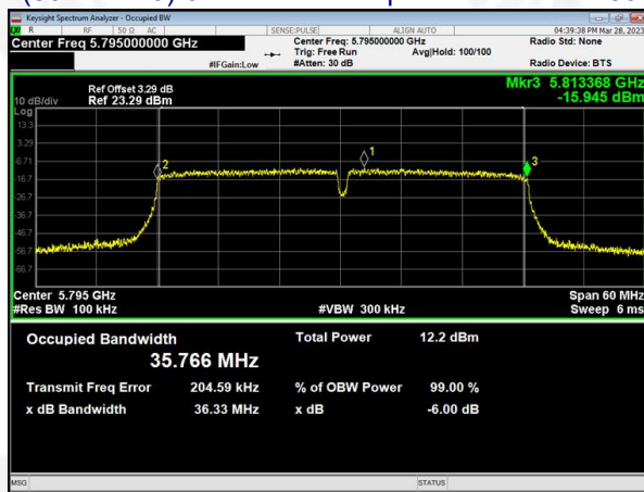
(802.11n40) 6dB Bandwidth plot on channel 159
