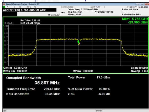
(802.11n40) 6dB Bandwidth plot on channel 151
