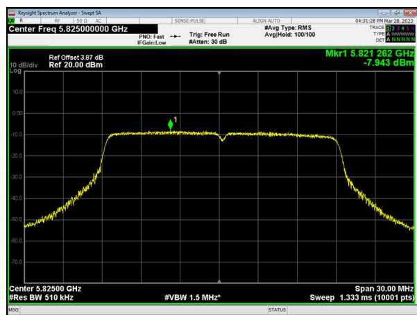
(802.11n20) PSD plot on channel 165
