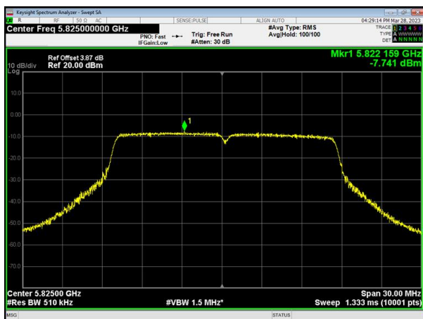
(802.11a) PSD plot on channel 165
