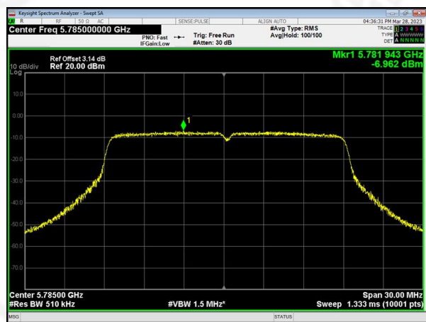
(802.11n20) PSD plot on channel 165
