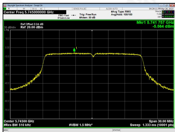
(802.11n20) PSD plot on channel 157
