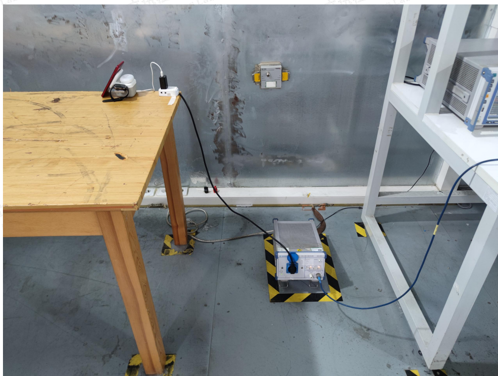
Conducted Emission-AC adapter charge mode
