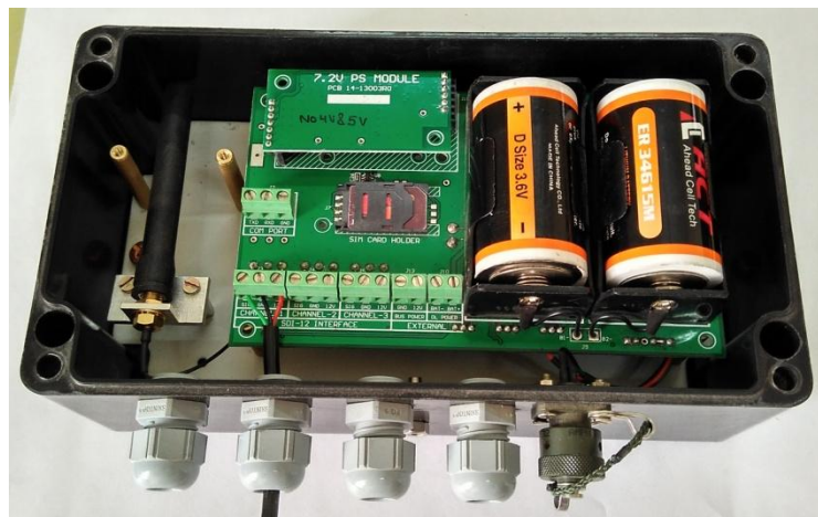
Figure 4-2 Datalogger powered with 2 x 3.6 V Lithium Batteries
