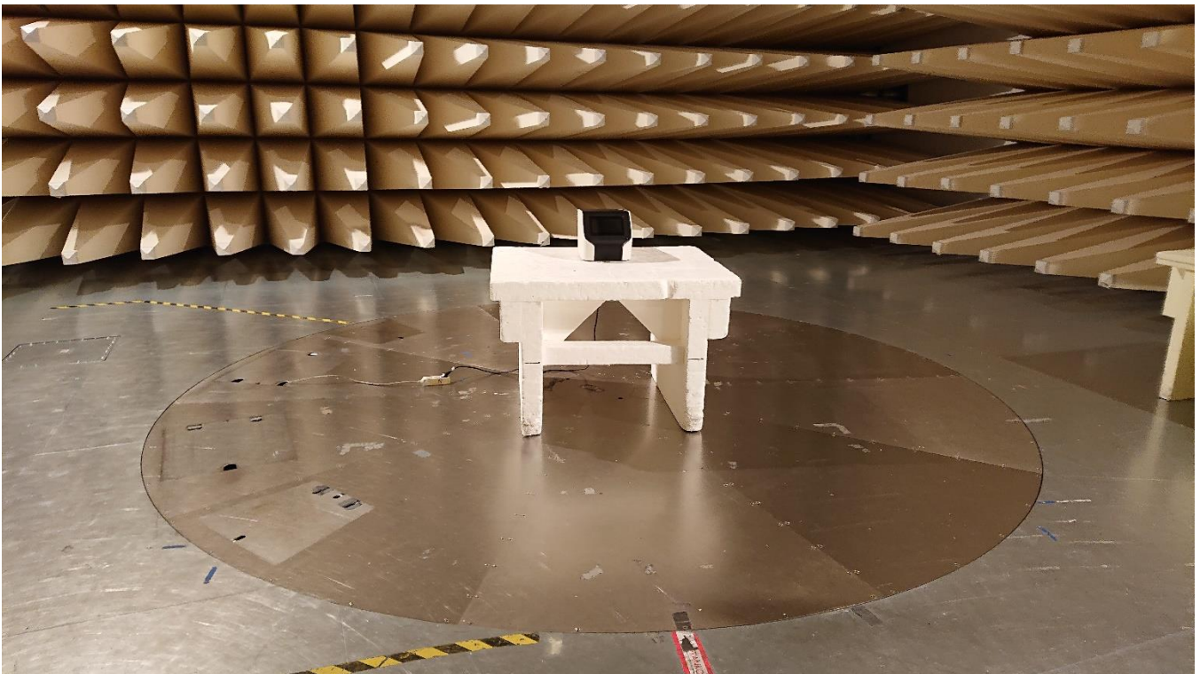
Photograph 4. Radiated Emissions 30 – 1000 MHz
