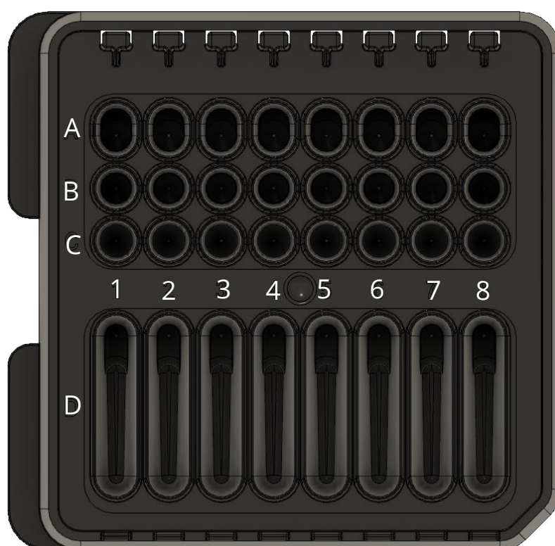
Fig. 3.1. dPCR cartridge top view with wells (A-D) and lanes (1-8) marked.
