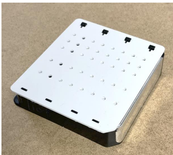
Fig. 3.4. The Xdrop DE20 Sort Cartridge covered with foil and the Xdrop DE20 Sort Gasket.
