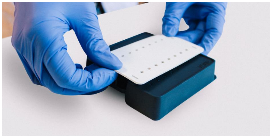
Fig. 5.4. Attach the white rubber Xdrop SE 85 Gasket to T-hooks of the Xdrop SE85 Cartridge. Note that a gasket should only be used once to avoid contamination.
