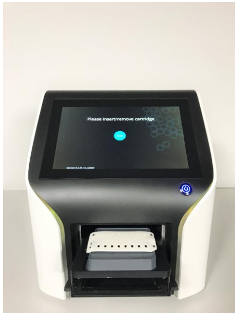
Fig. 5.6. Photo of Xdrop Sort with a correctly inserted Xdrop SE85 Cartridge.
