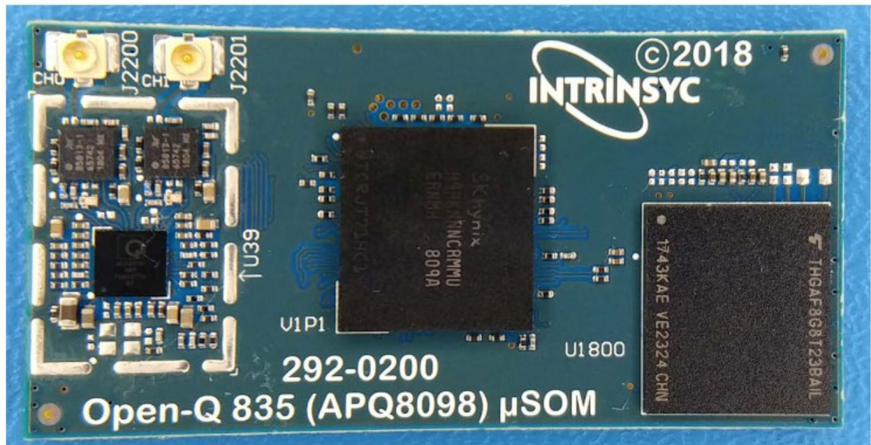
Figure 15: \mu SOM with Shielding removed
