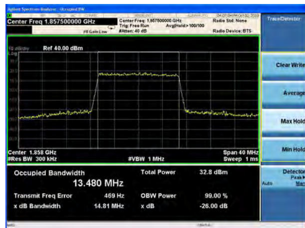
LTE Band 25 15MHz QPSK CH-Middle
