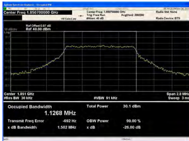
LTE Band 2 1.4MHz 64QAM CH-Middle
