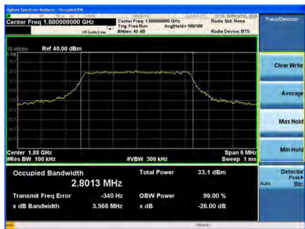
LTE Band 2 3MHz 16QAM CH-High
