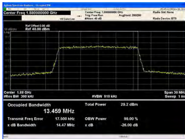
LTE Band 2 15MHz 64QAM CH-High
