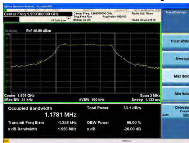
LTE Band 2 1.4MHz 16QAM CH-High
