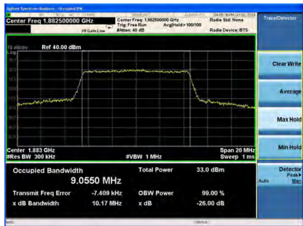
LTE Band 25 10MHz 16QAM CH-High
