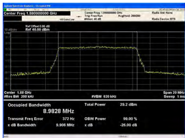
LTE Band 2 10MHz 64QAM CH-High
