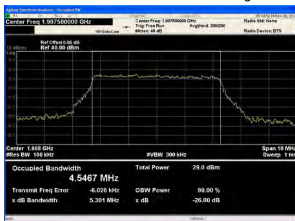
LTE Band 2 5MHz 64QAM CH-High
