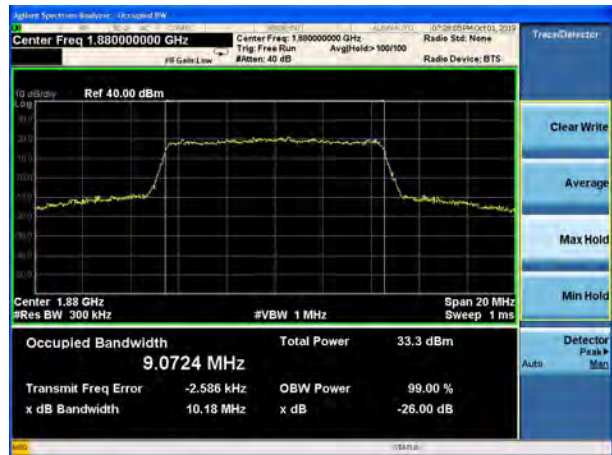
LTE Band 2 10MHz 16QAM CH-High
