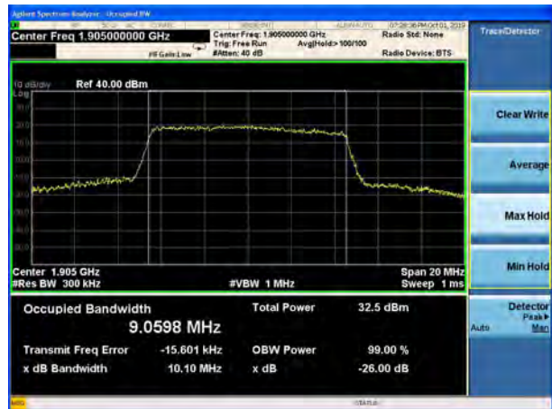
LTE Band 2 10MHz 16QAM CH-High
