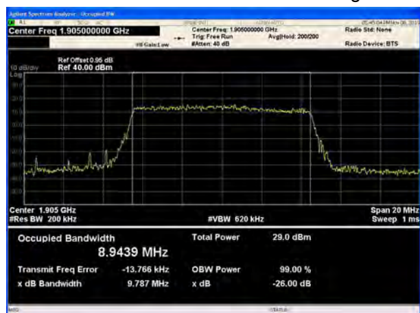
LTE Band 2 10MHz 64QAM CH-High
