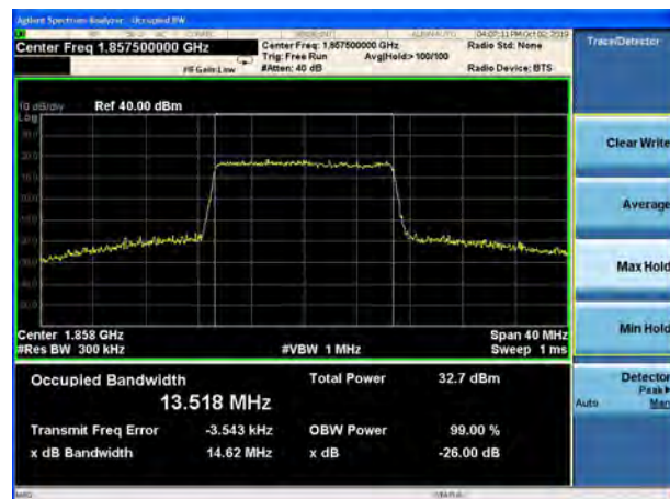
LTE Band 25 15MHz 16QAM CH-Middle
