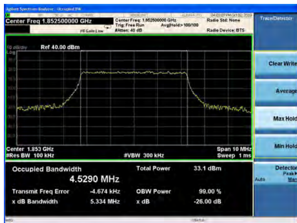
LTE Band 25 5MHz QPSK CH-Middle
