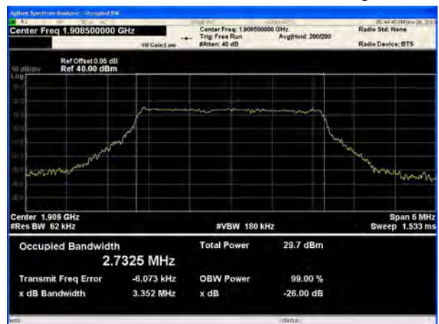
LTE Band 2 3MHz 64QAM CH-High
