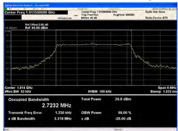
LTE Band 25 3MHz 64QAM CH-High
