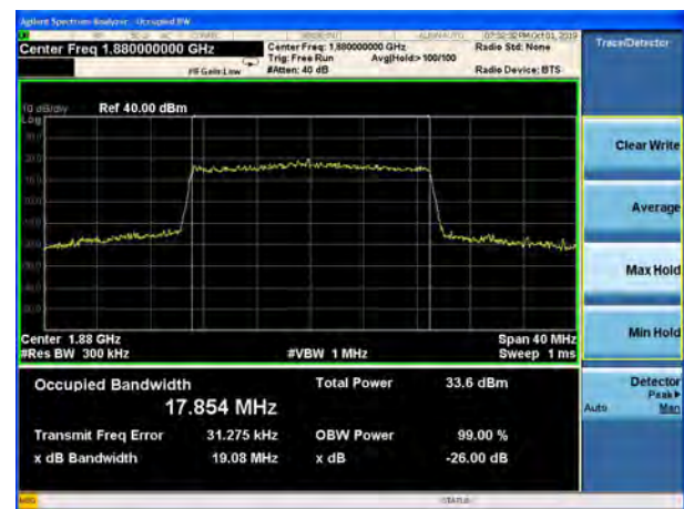
LTE Band 2 20MHz 16QAM CH-High
