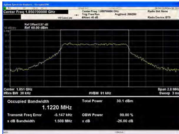
LTE Band 25 1.4MHz 64QAM CH-Middle
