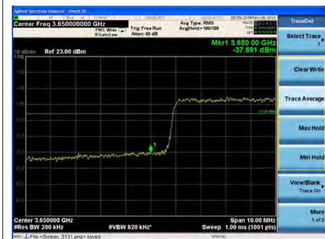
LTE Band 48 64QAM 20MHz CH-Low 100%RB
