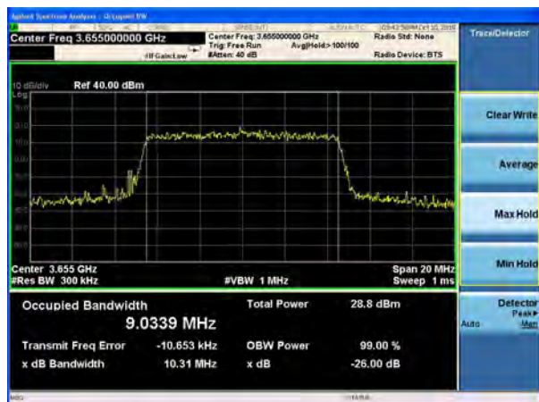
LTE Band 48 16QAM 10MHz CH-Middle
