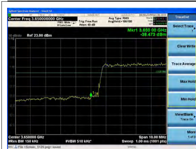
LTE Band 48 64QAM 20MHz CH-Low 1RB
