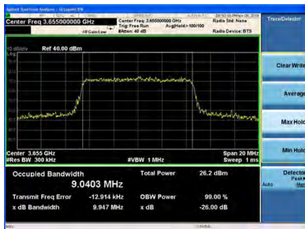
LTE Band 48 64QAM 10MHz CH-Middle
