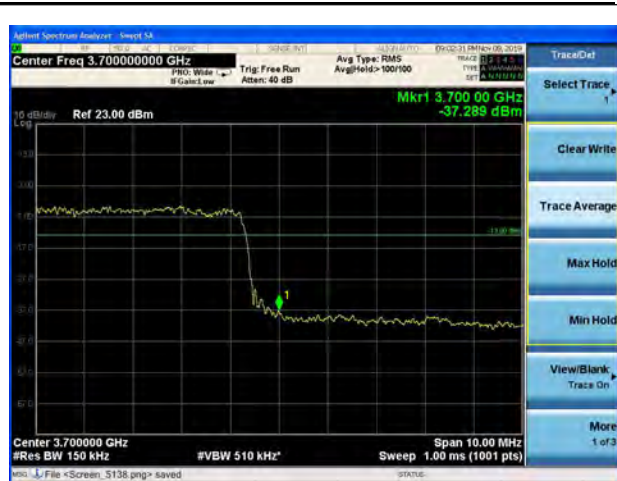
LTE Band 48 64QAM 20MHz CH-High 1RB
