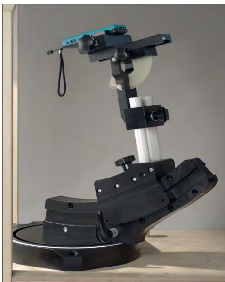
F-2. Device Holder for Transmitters
