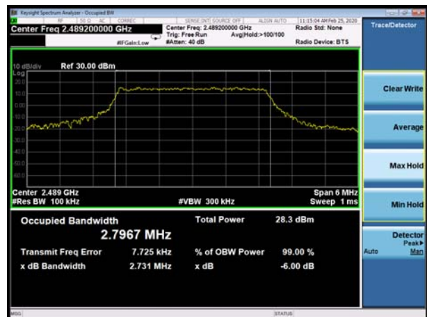
LTE Band 53 3MHz 64QAM CH-High
