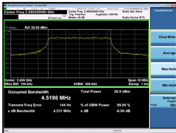
LTE Band 53 5MHz 64QAM CH-High
