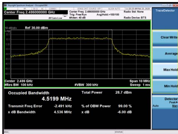
LTE Band 53 5MHz 64QAM CH-Middle
