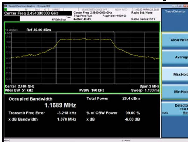
LTE Band 53 1.4MHz 64QAM CH-High
