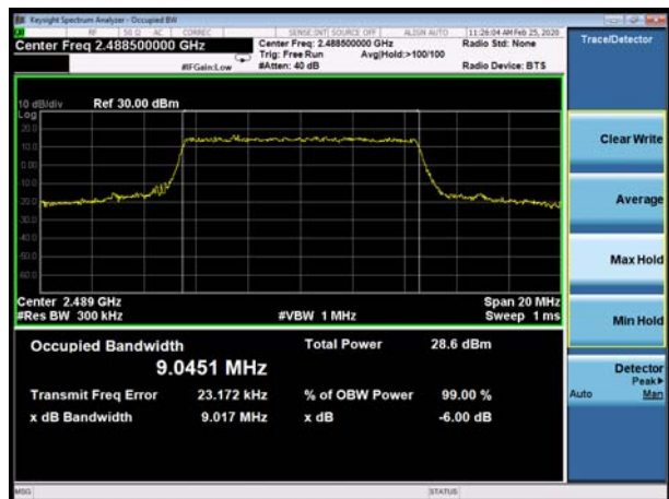
LTE Band 53 10MHz 64QAM CH-Middle
