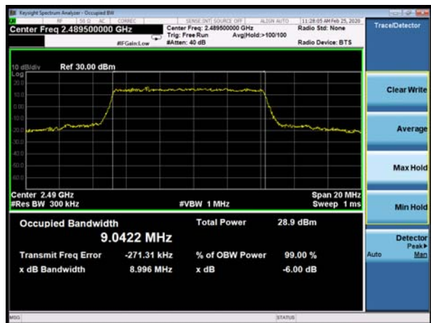
LTE Band 53 10MHz 64QAM CH-High
