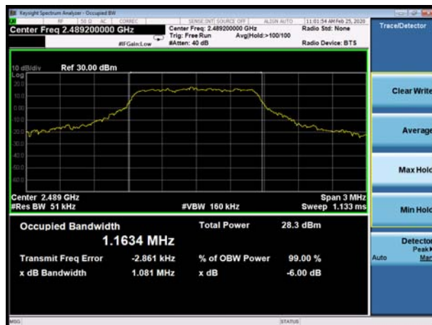
LTE Band 53 1.4MHz 64QAM CH-High
