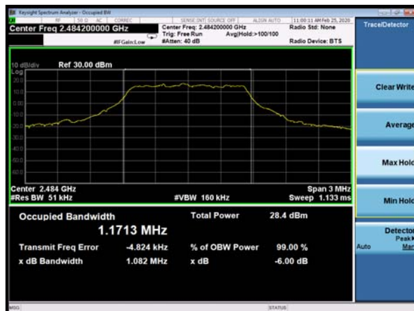
LTE Band 53 1.4MHz 64QAM CH-Middle
