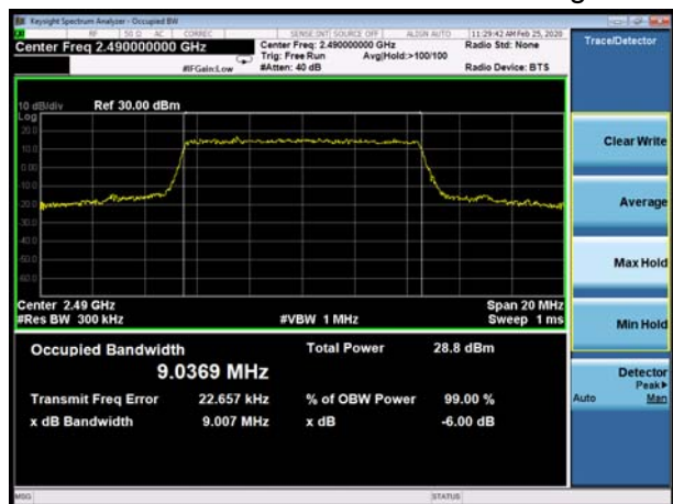
LTE Band 53 10MHz 64QAM CH-High
