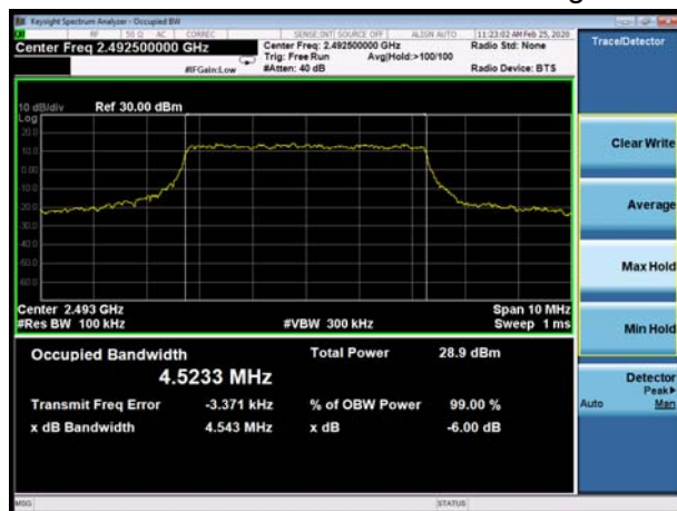
LTE Band 53 5MHz 64QAM CH-High
