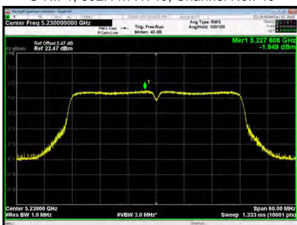
U-NII-1, 802.11ac VHT40, Channel No.: 38
