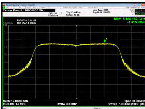
U-NII-1, 802.11ac VHT20, Channel No.: 40
