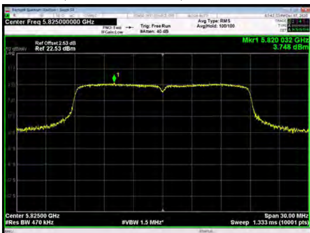
U-NII-3, 802.11ac VHT20, Channel No.: 165
