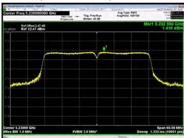
U-NII-1, 802.11ac VHT40, Channel No.: 46
