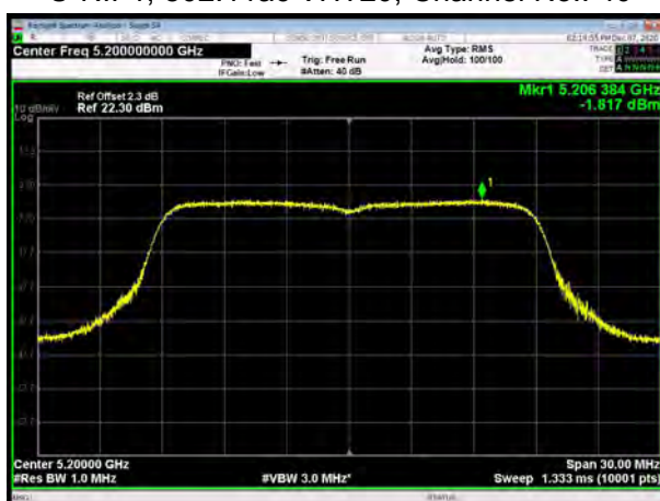
U-NII-1, 802.11ac VHT20, Channel No.: 48
