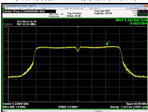
U-NII-1, 802.11ac VHT40, Channel No.: 38
