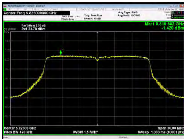
U-NII-3, 802.11ac VHT20, Channel No.: 165
