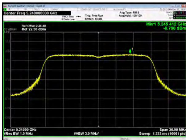
U-NII-1, 802.11ac VHT20, Channel No.: 48
