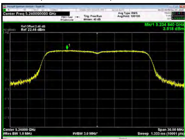
U-NII-1, 802.11ac VHT20, Channel No.: 48
