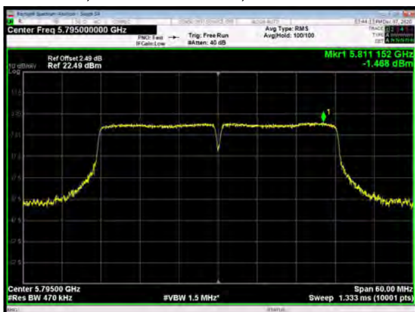
U-NII-3, 802.11ac VHT40, Channel No.: 159
