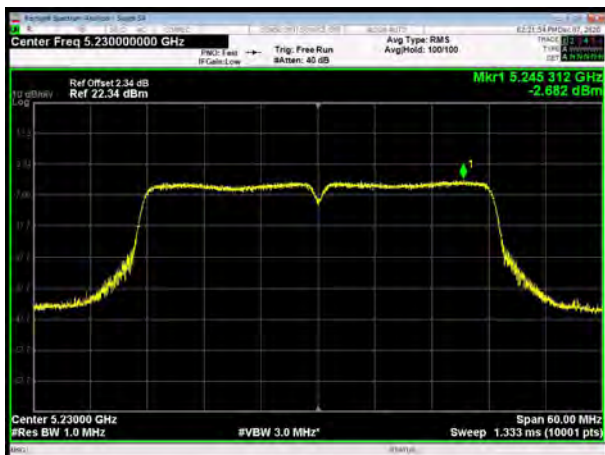
U-NII-1, 802.11ac VHT40, Channel No.: 46
