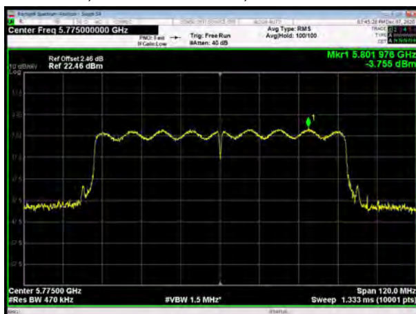
U-NII-3, 802.11ac VHT80, Channel No.: 155
