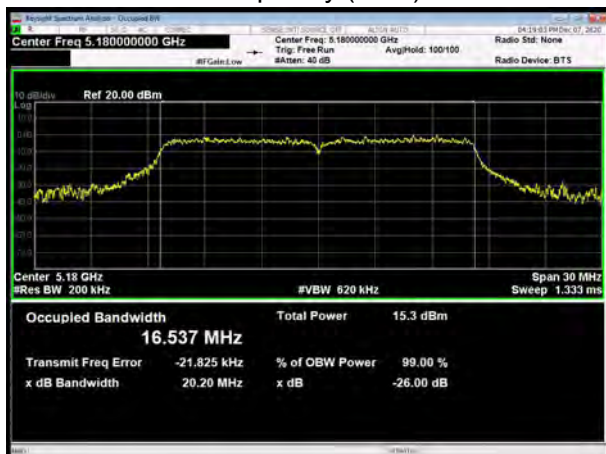
U-NII-1, 802.11a Carrier frequency (MHz): 5200
