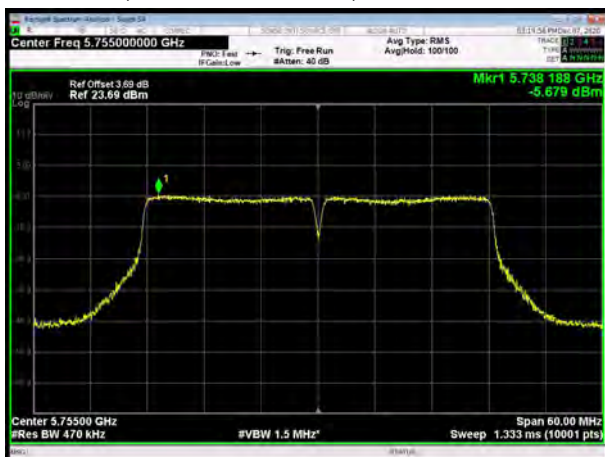
U-NII-3, 802.11ac VHT40, Channel No.: 151
