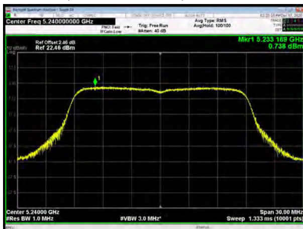
U-NII-1, 802.11ac VHT20, Channel No.: 48
