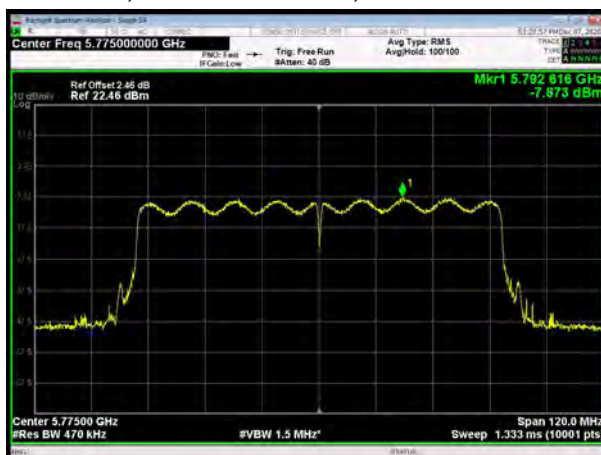
U-NII-3, 802.11ac VHT80, Channel No.: 155
