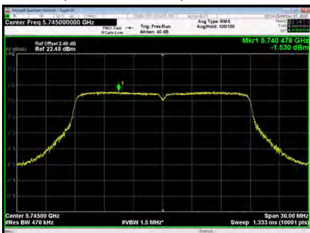
U-NII-3, 802.11ac VHT20, Channel No.: 157
