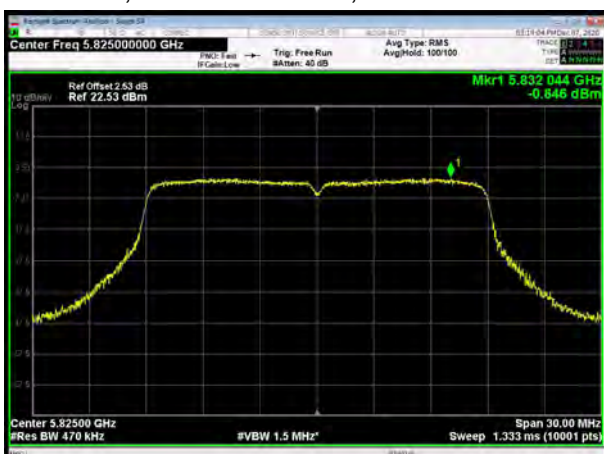
U-NII-3, 802.11ac VHT20, Channel No.: 165
