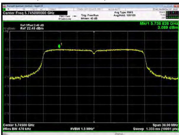
U-NII-3, 802.11ac VHT20, Channel No.: 157
