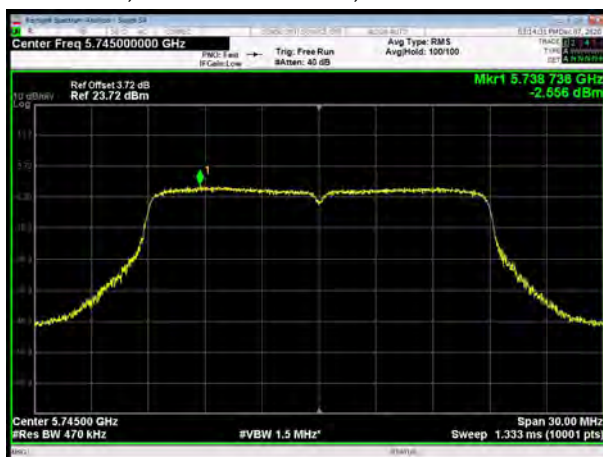
U-NII-3, 802.11ac VHT20, Channel No.: 157
