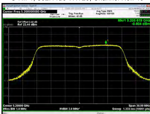
U-NII-1, 802.11ac VHT20, Channel No.: 48
