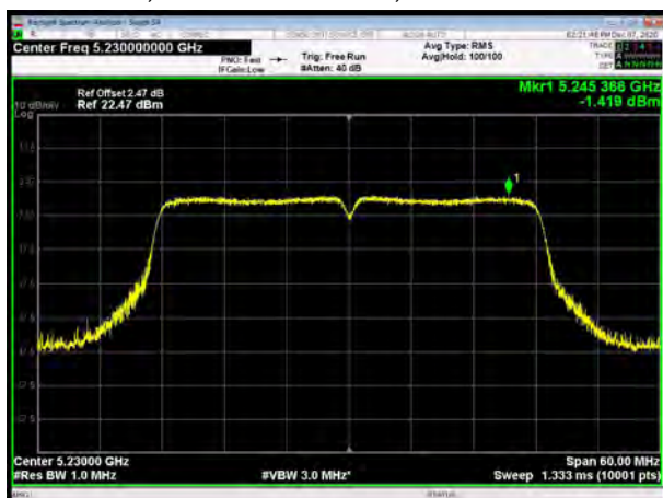
U-NII-1, 802.11ac VHT40, Channel No.: 46
