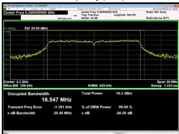
U-NII-1, 802.11a Carrier frequency (MHz): 5240
