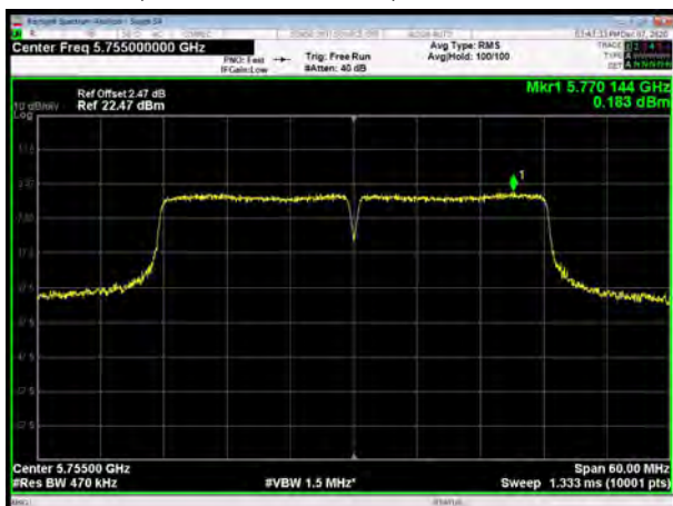
U-NII-3, 802.11ac VHT40, Channel No.: 151
