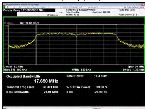
U-NII-1, 802.11n HT20 Carrier frequency (MHz): 5240
