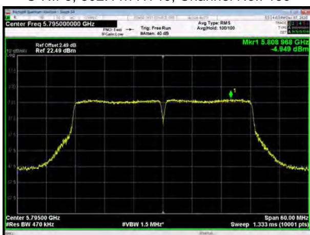
U-NII-3, 802.11ac VHT40, Channel No.: 151
