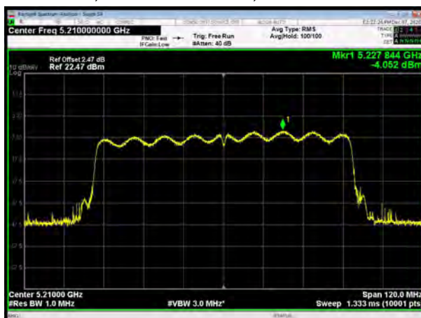
U-NII-1, 802.11ac VHT80, Channel No.: 42
