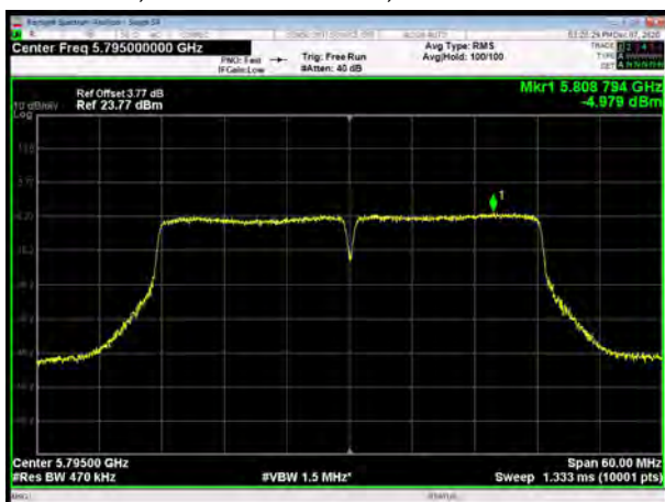
U-NII-3, 802.11ac VHT40, Channel No.: 159
