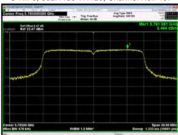
U-NII-3, 802.11ac VHT20, Channel No.: 165
