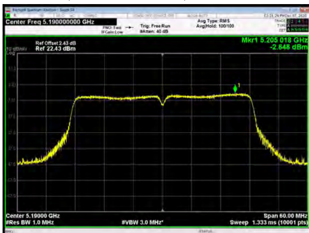
U-NII-1, 802.11ac VHT40, Channel No.: 38
