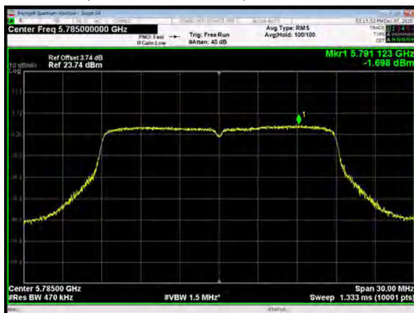
U-NII-3, 802.11ac VHT20, Channel No.: 165
