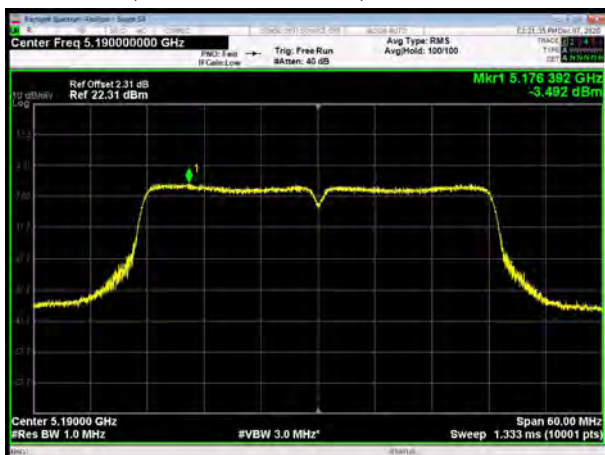
U-NII-1, 802.11ac VHT40, Channel No.: 38
