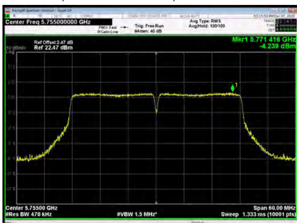
U-NII-3, 802.11ac VHT40, Channel No.: 151
