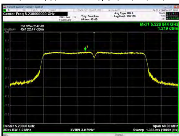
U-NII-1, 802.11ac VHT40, Channel No.: 38
