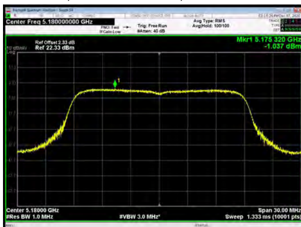
U-NII-1, 802.11ac VHT20, Channel No.: 40
