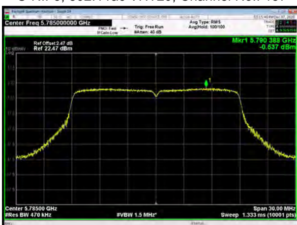
U-NII-3, 802.11ac VHT20, Channel No.: 165
