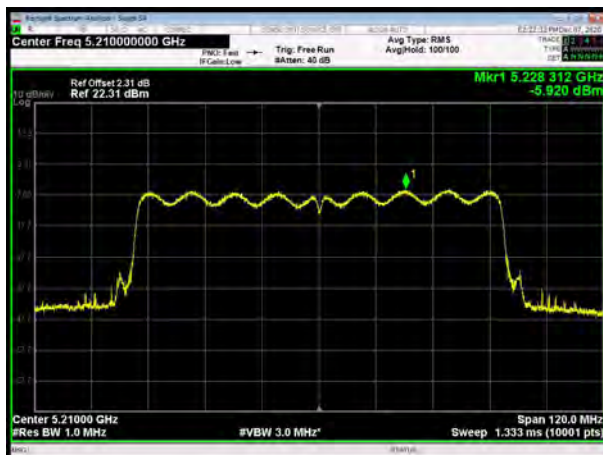
U-NII-1, 802.11ac VHT80, Channel No.: 42
