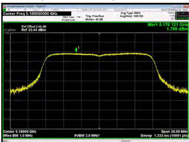
U-NII-1, 802.11ac VHT20, Channel No.: 40
