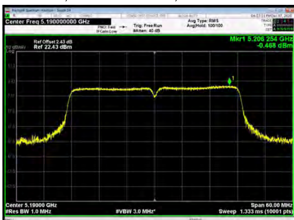
U-NII-1, 802.11ac VHT40, Channel No.: 38
