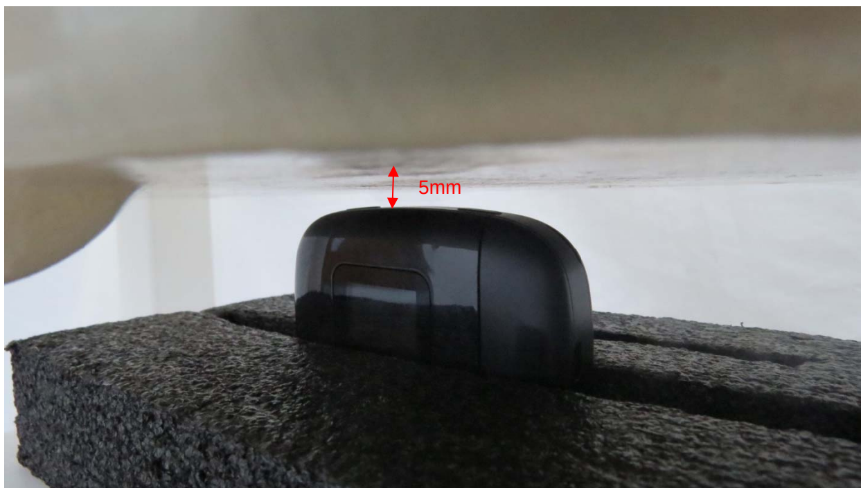
Picture 4: Right Side, the distance from handset to the bottom of the Phantom is 5mm
