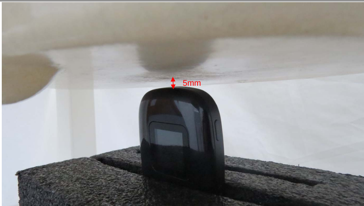
Picture 5: Top Side, the distance from handset to the bottom of the Phantom is 5mm
