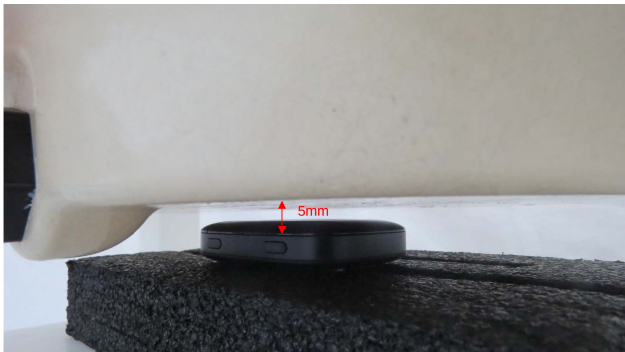
Picture 2: Front Side, the distance from handset to the bottom of the Phantom is 5mm
