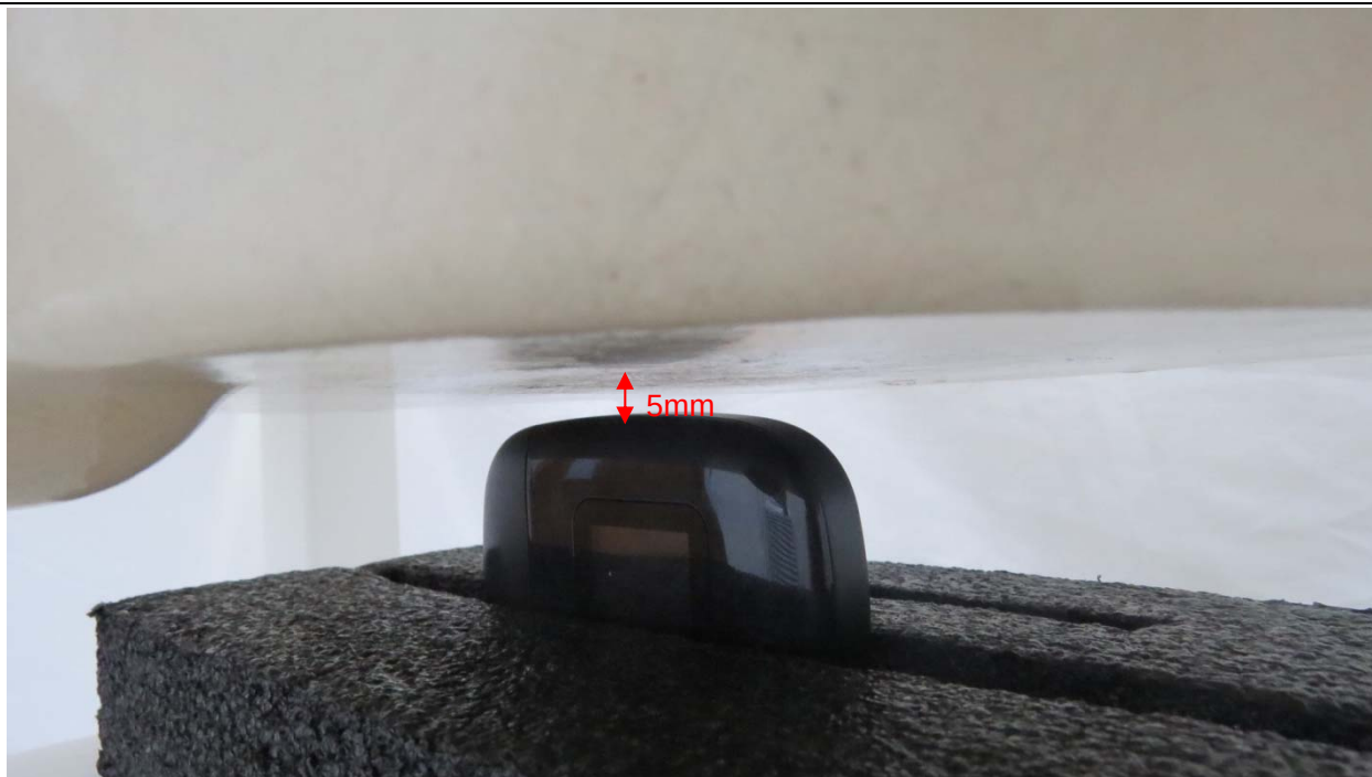
Picture 3: Left Side, the distance from handset to the bottom of the Phantom is 5mm
