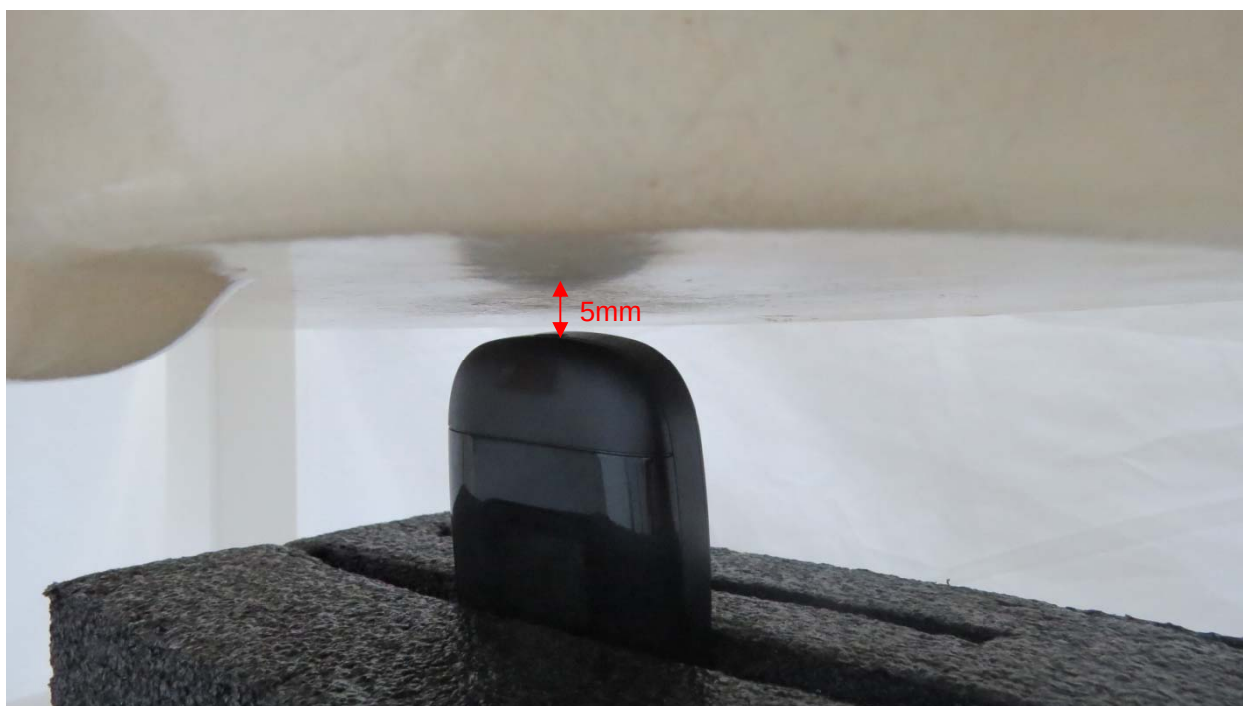
Picture 6: Bottom Edge, the distance from handset to the bottom of the Phantom is 5mm
