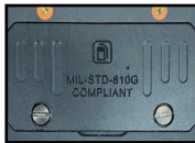
Figure 4 Close the back cover of the SIM card
