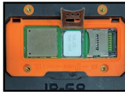
Figure 2 Put the SIM card into the card slot
