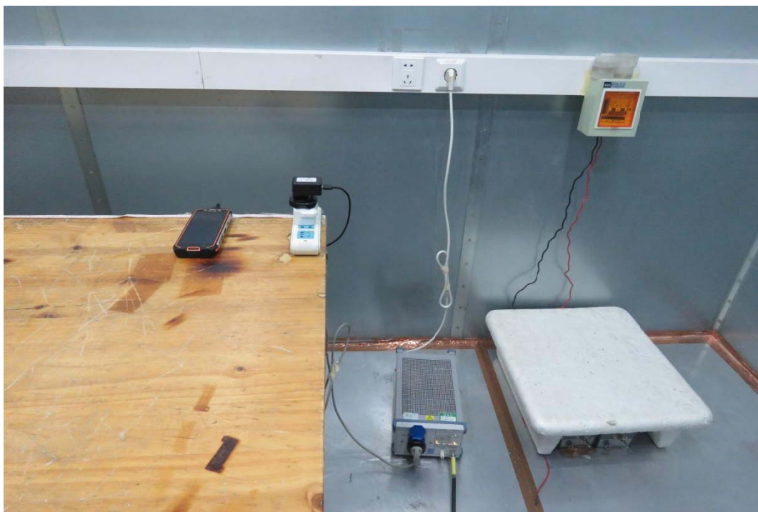
Picture 2 Conducted Emission Test Setup
