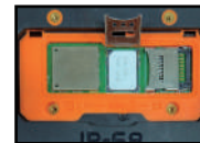
Figure 2 Put the SIM card into the card slot
