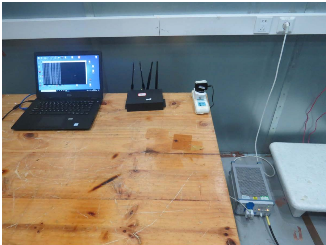
Picture 2 Conducted Emission Test Setup
