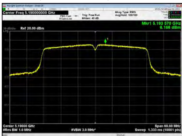
U-NII-1, 802.11ac VHT40, Channel No.: 38
