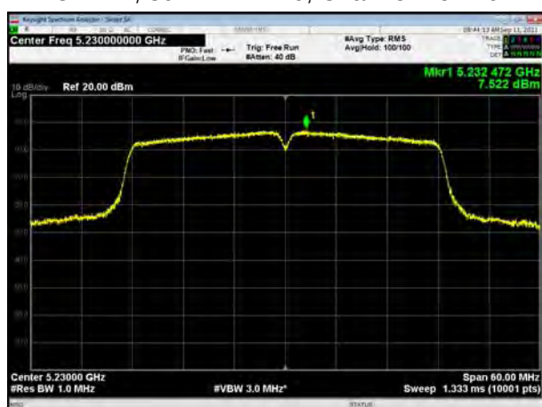
U-NII-1, 802.11ac VHT40, Channel No.: 38
