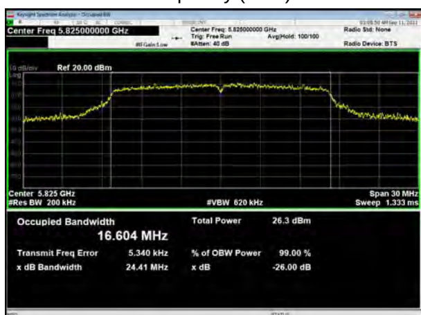
U-NII-3, 802.11a Carrier frequency (MHz): 5825
