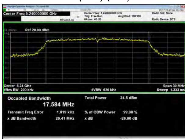
U-NII-1, 802.11n HT20 Carrier frequency (MHz): 5240
