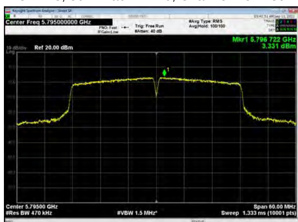
U-NII-3, 802.11ac VHT40, Channel No.: 159
