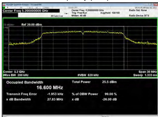
U-NII-1, 802.11a Carrier frequency (MHz): 5240
