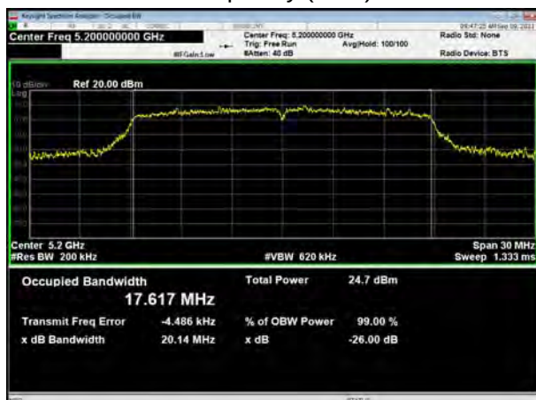
U-NII-1, 802.11n HT20 Carrier frequency (MHz): 5240
