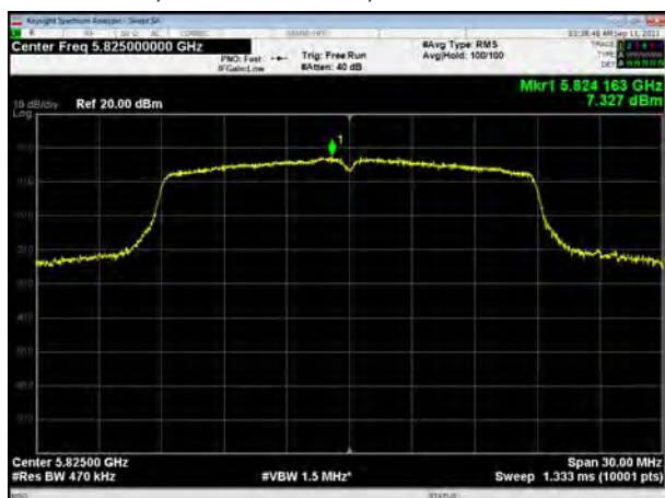
U-NII-3, 802.11ac VHT20, Channel No.: 149
