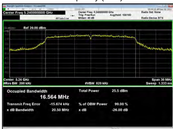
U-NII-1, 802.11a Carrier frequency (MHz): 5240
