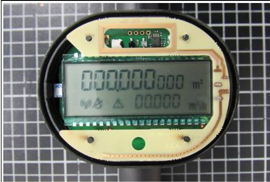
EUT Housing Open, antenna View
