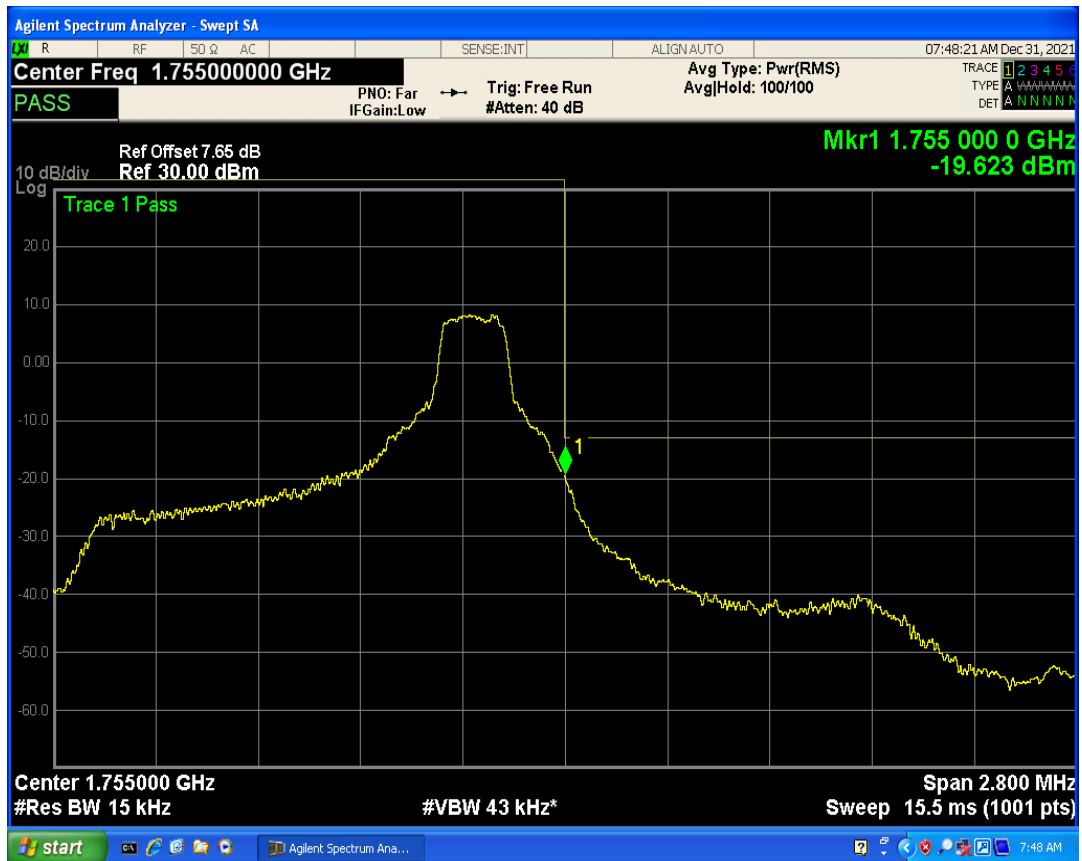
Band4 QAM16 BW=1.4MHz Channel=20393 RB Size=1 Position=#0
