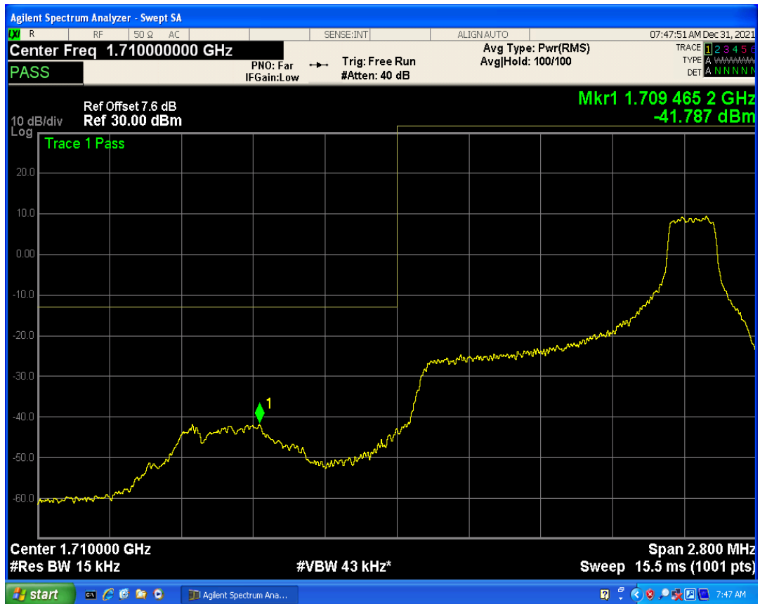
Band4 QAM16 BW=1.4MHz Channel=19957 RB Size=1 Position=#0
