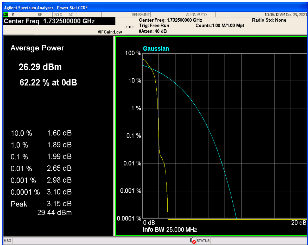
Band4 QAM16 BW=20MHz Channel=20175 RB Size=1 Position=#0
