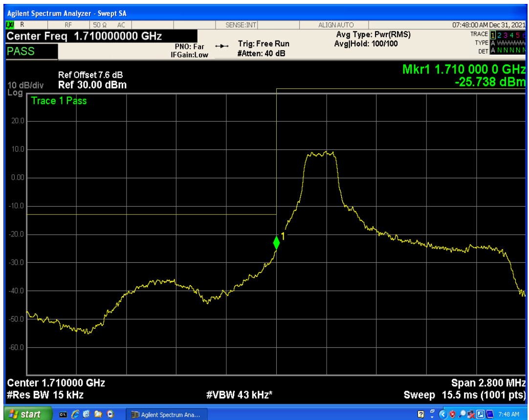
Band4 QPSK BW=1.4MHz Channel=19957 RB Size=6 Position=#0
