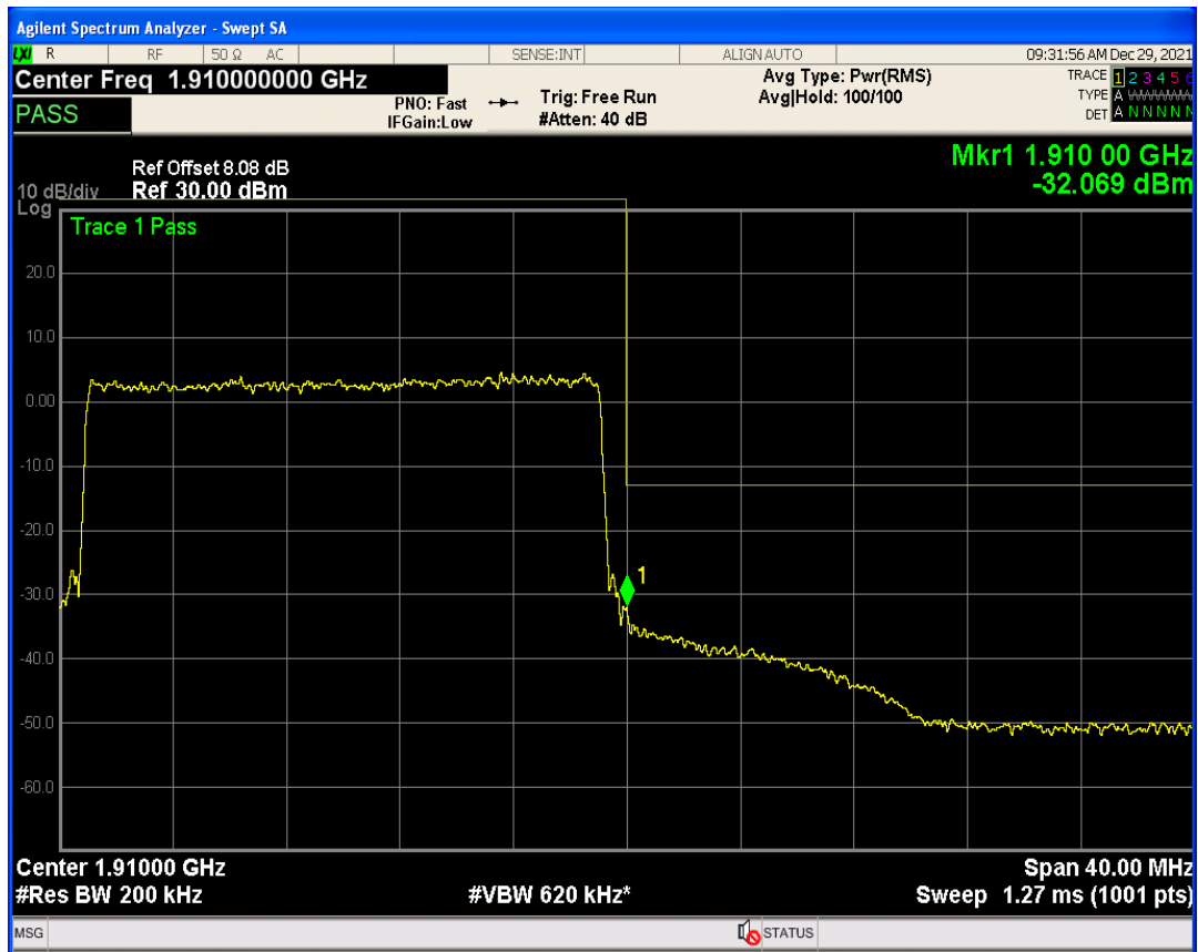
Band2 QAM16 BW=20MHz Channel=19100 RB Size=100 Position=#0
