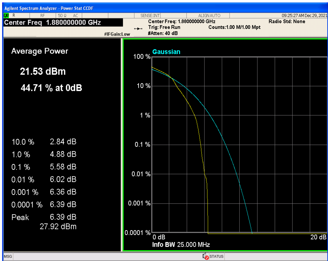
Band2 QPSK BW=10MHz Channel=18900 RB Size=1 Position=#0
