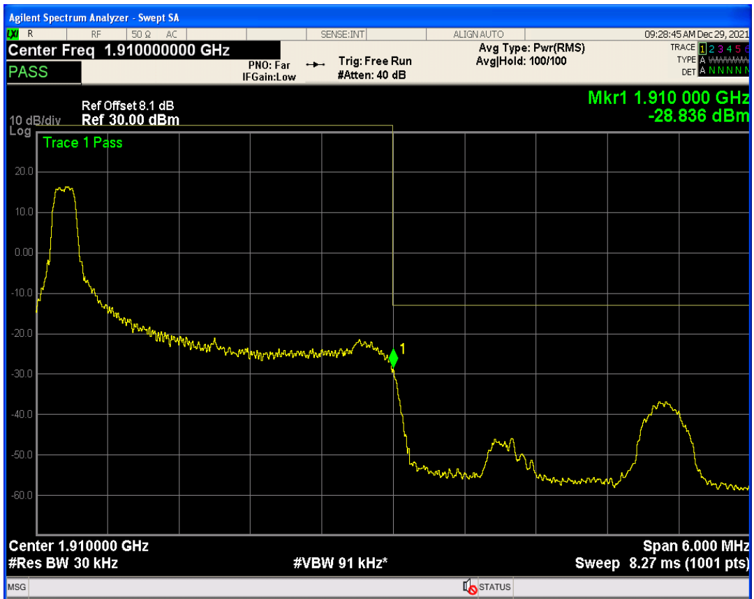
Band2 QPSK BW=3MHz Channel=19185 RB Size=15 Position=#0
