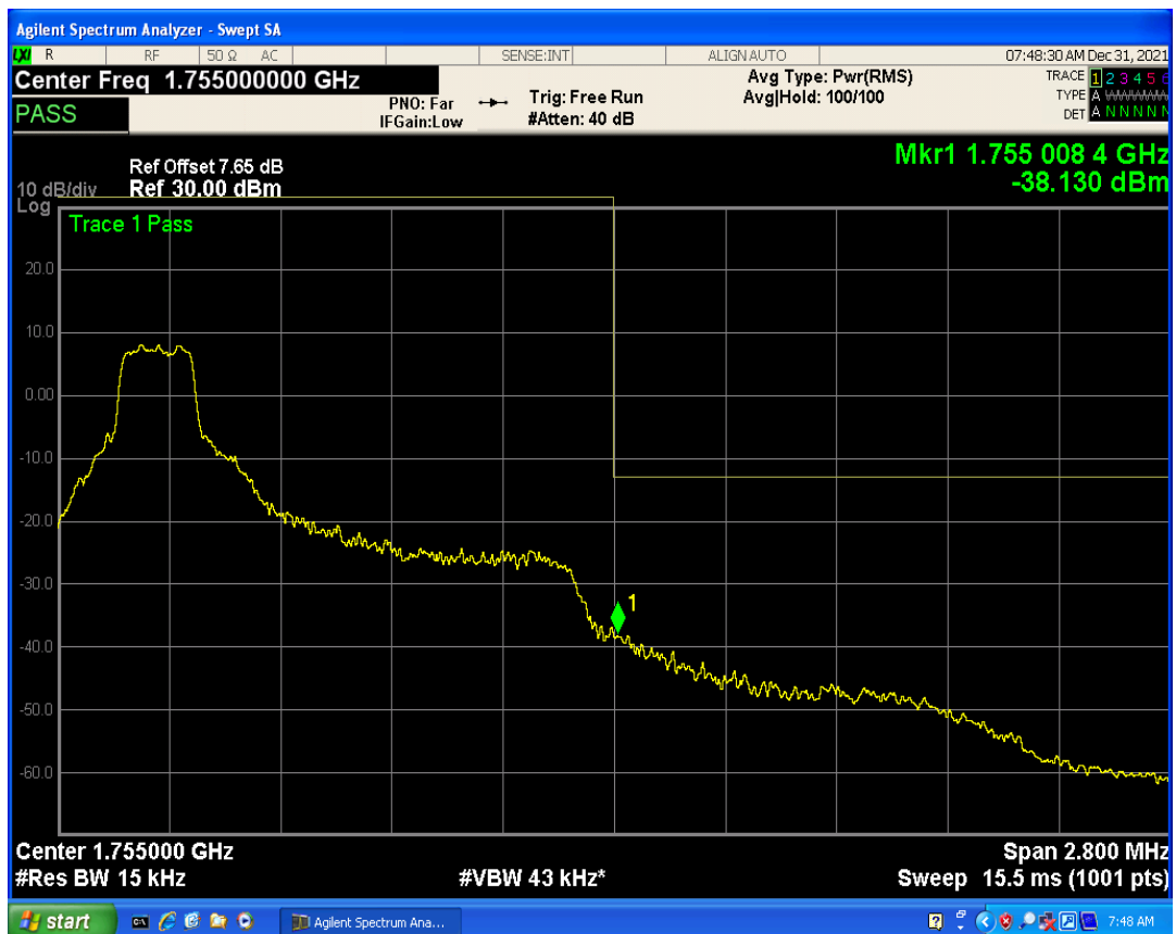
Band4 QPSK BW=1.4MHz Channel=20393 RB Size=6 Position=#0
