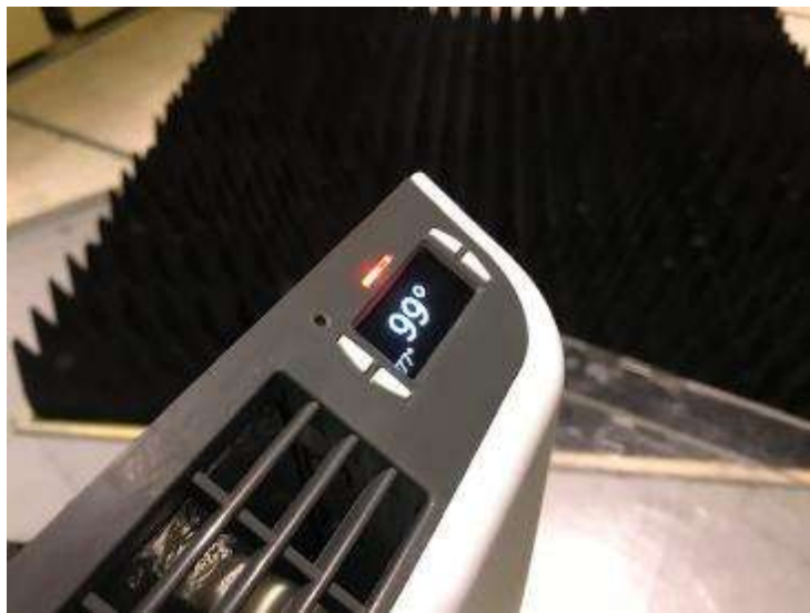
Location of transceiver and antenna is behind LCD display. This places the transceiver at the required 150 cm height.
