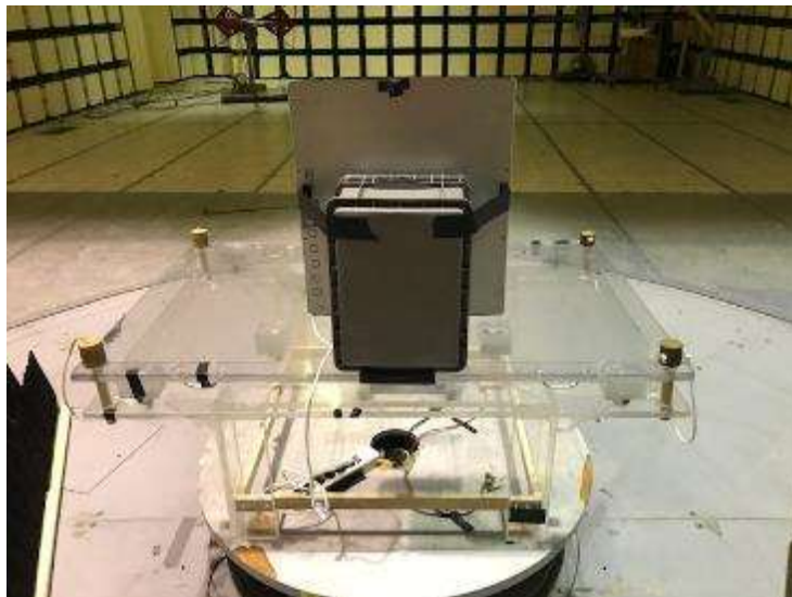
Radiated Emissions, Back, Below 1 GHz
