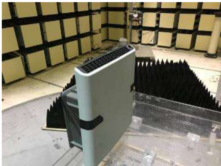
Radiated Emissions, 1 to 18 GHz
