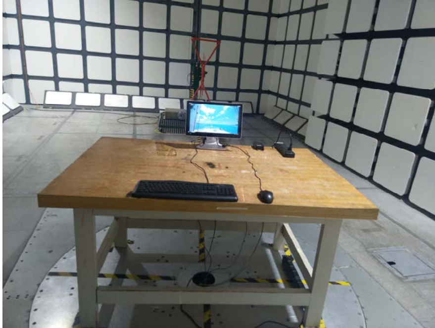
Radiated Emissions – Front View (Below 1 GHz)
