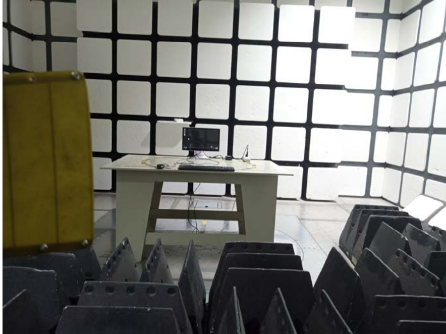
Radiated Emissions – Front View (Above 1 GHz)
