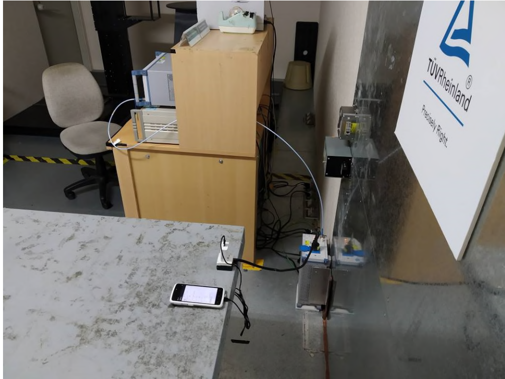
Photograph 6: Set-up for for AC Mains (Front)
