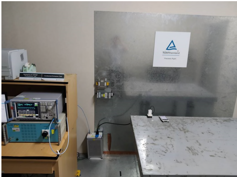
Photograph 6: Set-up for for AC Mains (Front)
