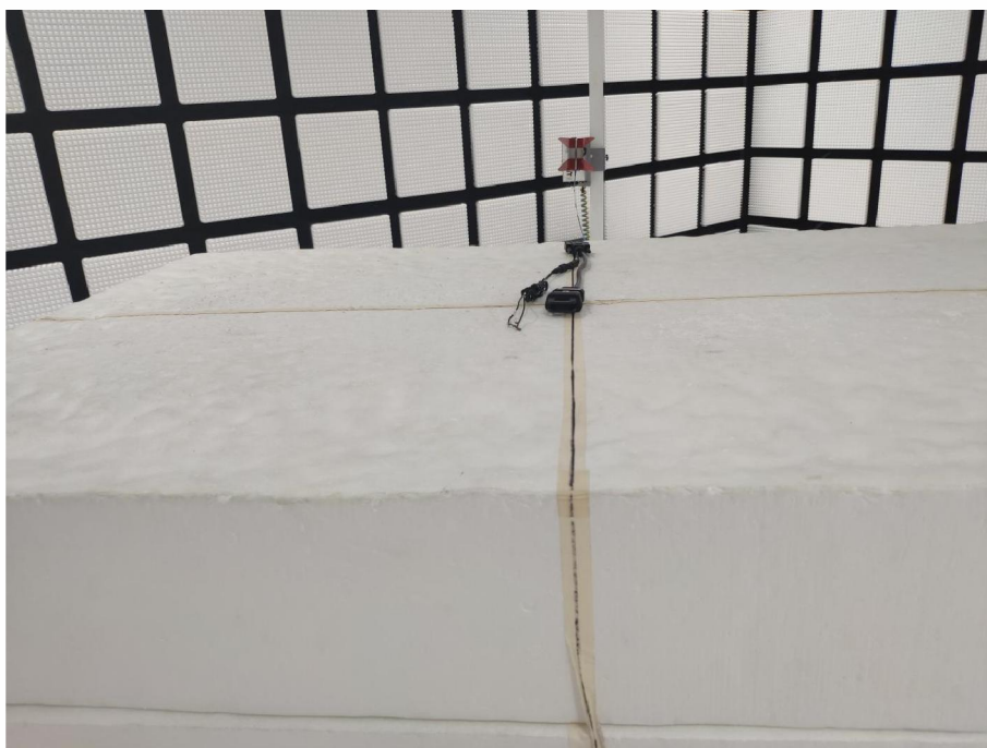
Radiated spurious emission Test Setup-3(Above 1GHz)
