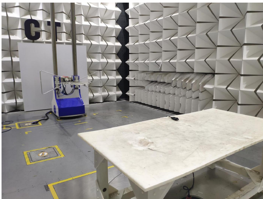
Radiated spurious emission Test Setup-2(Below 1GHz)
