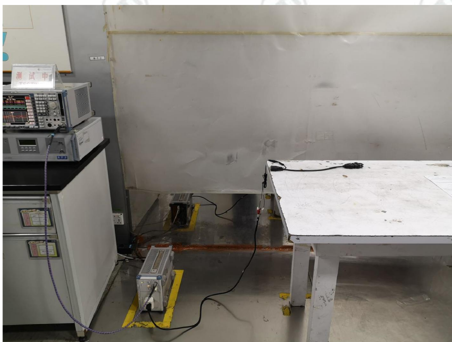
Conducted Emissions Test Setup
