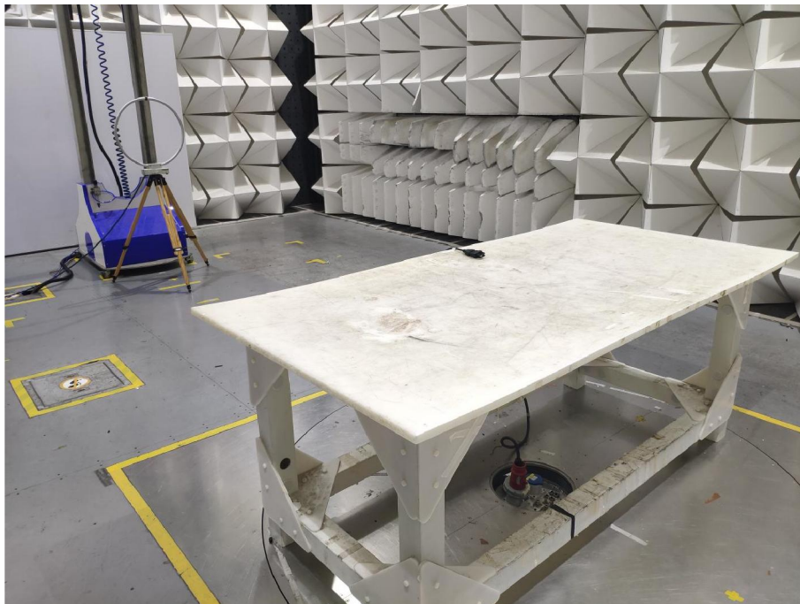
Radiated spurious emission Test Setup-1(Below 30MHz)
