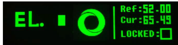
Figure 5-3-1-8: Elevation angle fine-tune is completed
