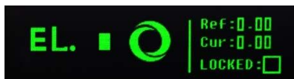
Figure 5-3-1-2: Elevation angle coarse adjustment is completed
