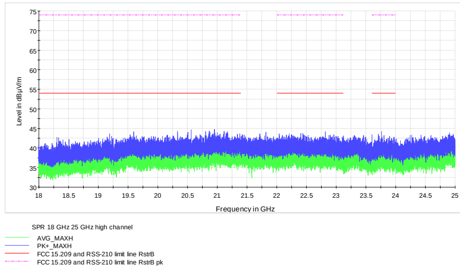
Figure 7.6-11: radiated spurious emissions from 18 GHz to 25 GHz on 802.11b (1 Mbps) at high channel
