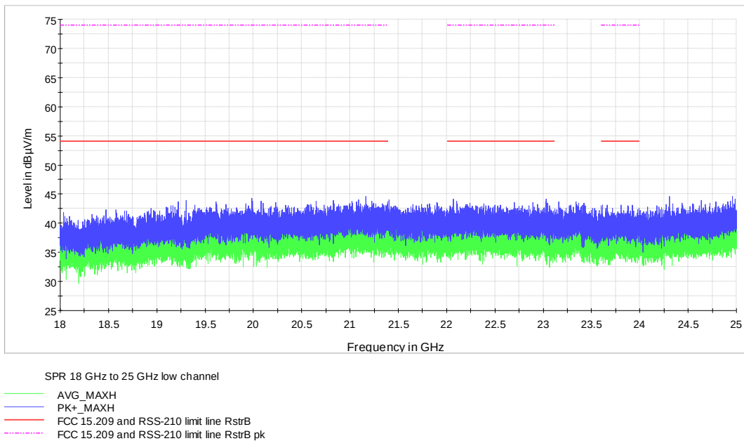
Figure 7.6-9: radiated spurious emissions from 18 GHz to 25 GHz on 802.11b (1 Mbps) at low channel
