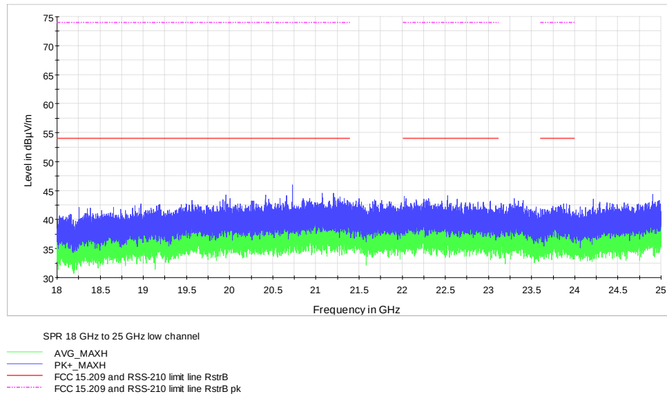
Figure 7.6-35: radiated spurious emissions from 18 GHz to 25 GHz on 802.11g (6 Mbps) at low channel
