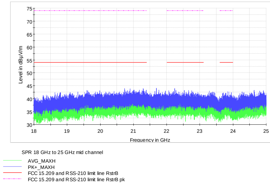
Figure 7.6-23: radiated spurious emissions from 18 GHz to 25 GHz on 802.11b (11 Mbps) at mid channel
