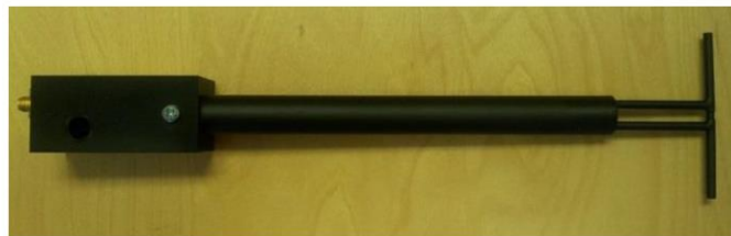
Figure 1 – MVG COMOSAR Validation Dipole
